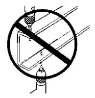
FIGURE 4-8. Frame Rail Flange Drilling Prohibited
