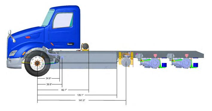
FIGURE 3-2b. 579 BEV Dimensions 216" (shown with optional ePTO)
