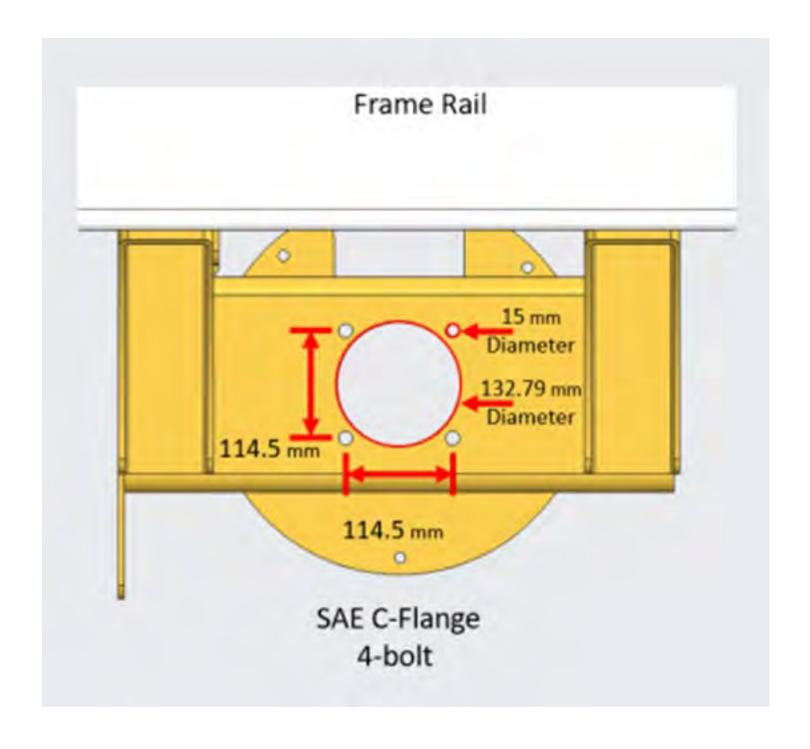
FIGURE 7-4. Mounting Surface for Hydraulic Pump (View from underneath frame looking outward to backside of ePTO)
