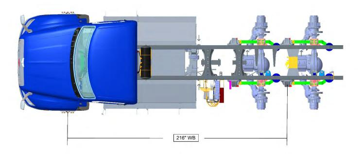
FIGURE 3-3a. 579 BEV 216" Wheelbase (shown with optional ePTO)
