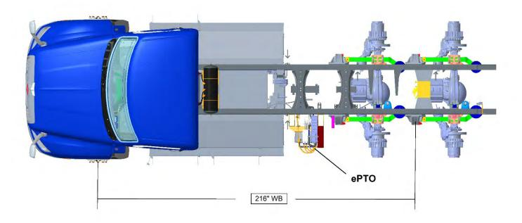
FIGURE 7-1. Model 579 BEV with ePTO mount
