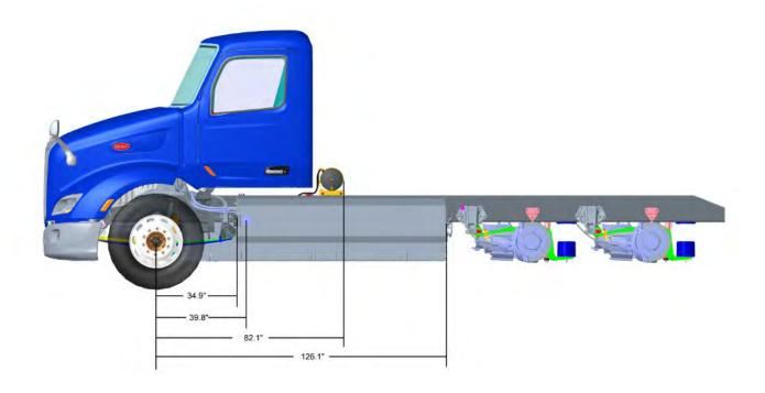
FIGURE 3-2a. 579 BEV Dimensions 190" WB
