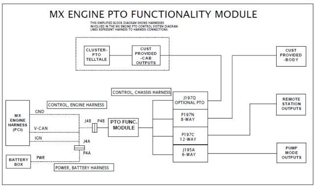
FIGURE 6-15. Optional PTO Module Block Diagram
