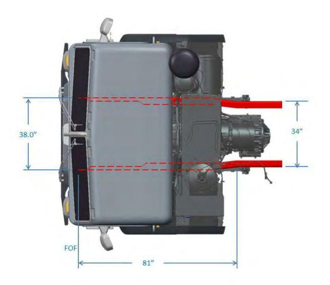
FIGURE 3-9. Model 520 Frame Rail
