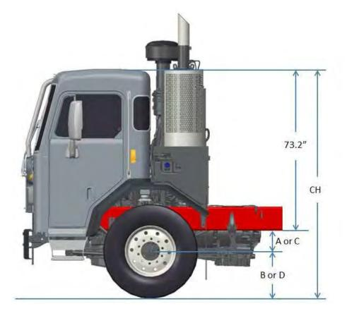
FIGURE 3-30. Overall Cab Height Calculations
