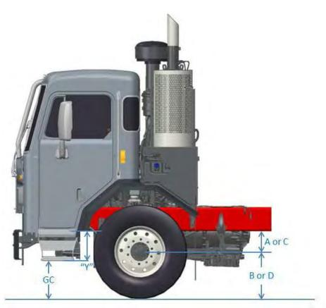
FIGURE 3-28. Ground Clearance Calculations
