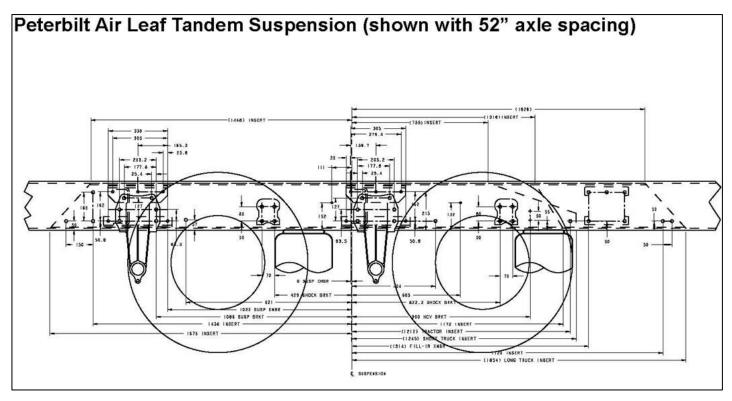
FIGURE 3-9. Peterbilt Air Leaf Tandem Frame Drilling (Dimensions In Millimeters)
