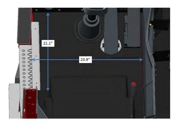
FIGURE 3-6. Floor Dimensions for LH Floor
