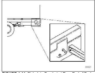
FIGURE 4-11. Fishplate Bracket at Rear End of Body
