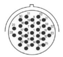
Figure 6-9. Cab Body Builder Connection 1 Pin Assignment
