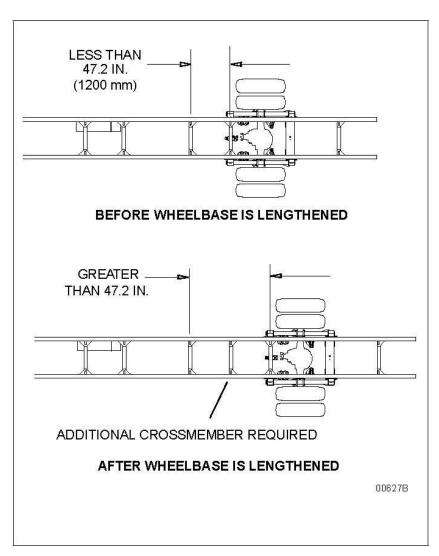
FIGURE 5-2. Crossmember Spacing Requirements
