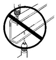
FIGURE 4-8. Frame Rail Flange Drilling Prohibited
