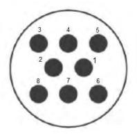
Figure 6-7. Cab Body Builder Connection 1 Pin Assignment
