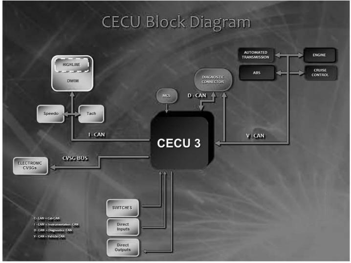
FIGURE 6-2. CECU Block Diagram
