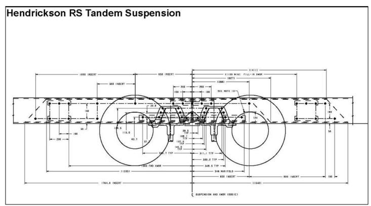
FIGURE 3-19. Hendrickson RS Tandem Frame Drilling (Dimensions In Millimeters)
