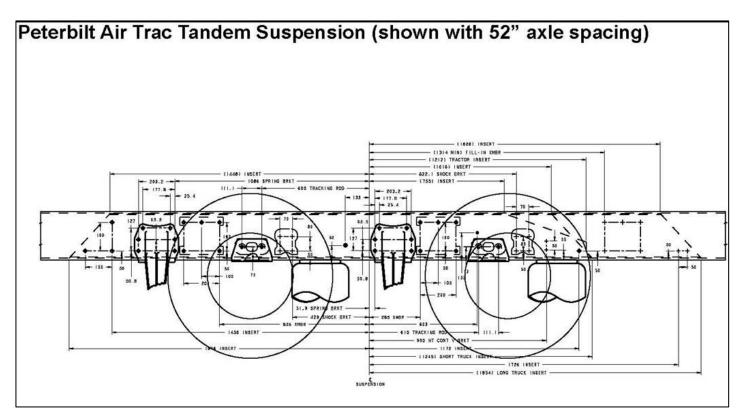
FIGURE 3-11. Peterbilt Air Trac Tandem Frame Drilling (Dimensions In Millimeters)
