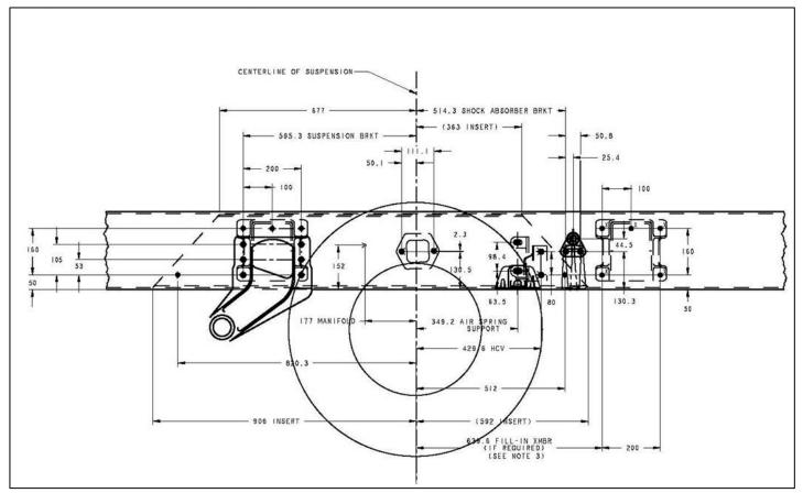
FIGURE 3-6. Reyco 102AR Frame Drilling (Dimensions In Millimeters)
