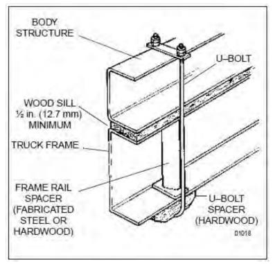
FIGURE 4-9. Acceptable U-Bolt Mounting with Wood and Fabricated Spacers
