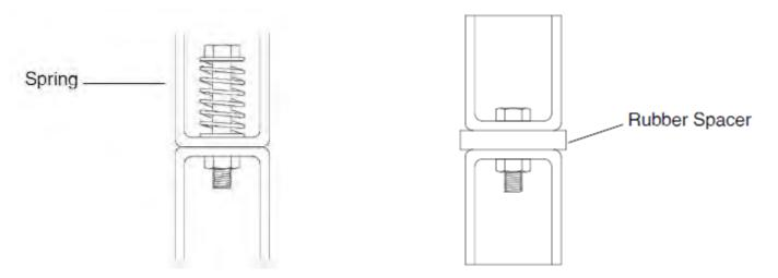
FIGURE 4-4. Mounting Brackets
