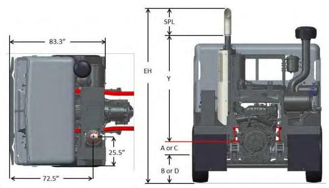
FIGURE 3-27. Exhaust Height Calculations
