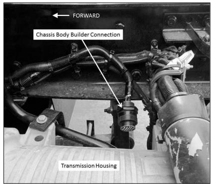
FIGURE 6-13. Chassis Body Builder Interface Location
