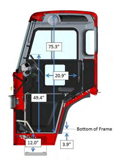
FIGURE 3-4. View Looking Through the Cab At The RH Drive Standup Version
