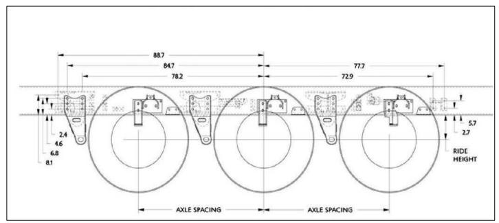
FIGURE 3-8. Neway ADZ 369/378 Frame Drilling (Dimensions In Millimeters)
