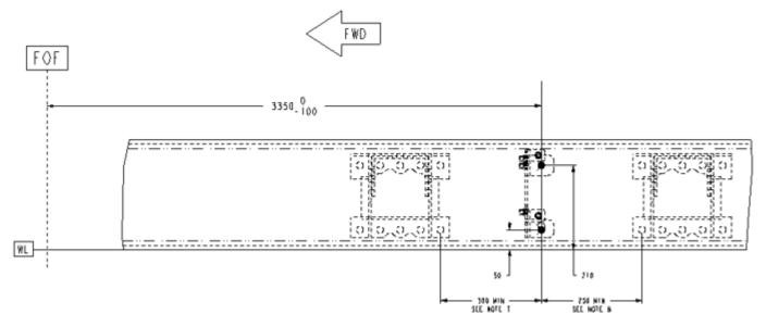
FIGURE 7-13. Optional Module Drilling Location for Bracket Installation
