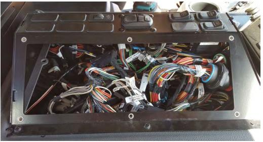
FIGURE 6-5. Body Builder Connections in Cab
