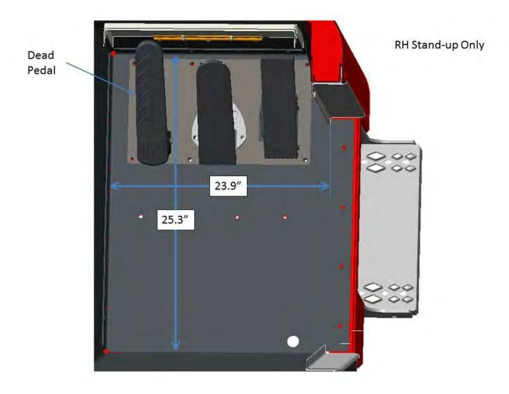
FIGURE 3-7. Passenger Floor RH Stand Up
