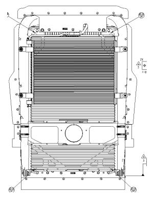
FIGURE 7-5. Cooling Module With FEPTO Provision
