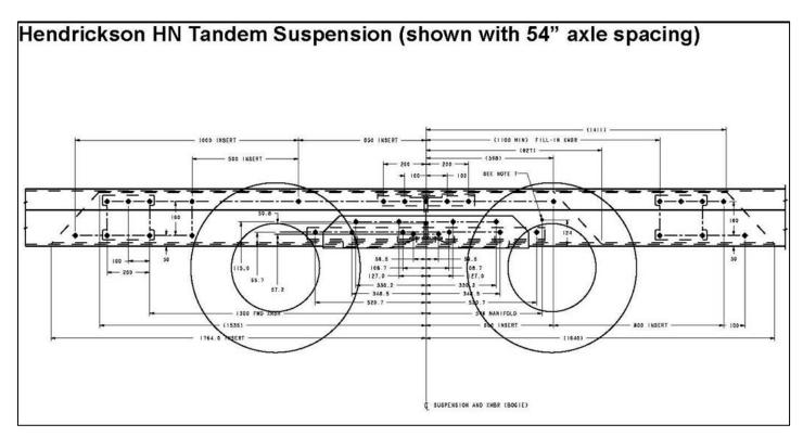
FIGURE 3-17. Hendrickson HN Tandem Frame Drilling (Dimensions In Millimeters)
