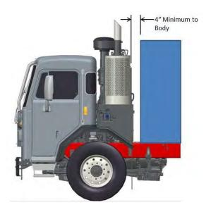
FIGURE 4-2. Minimum Back of Cab Clearance
