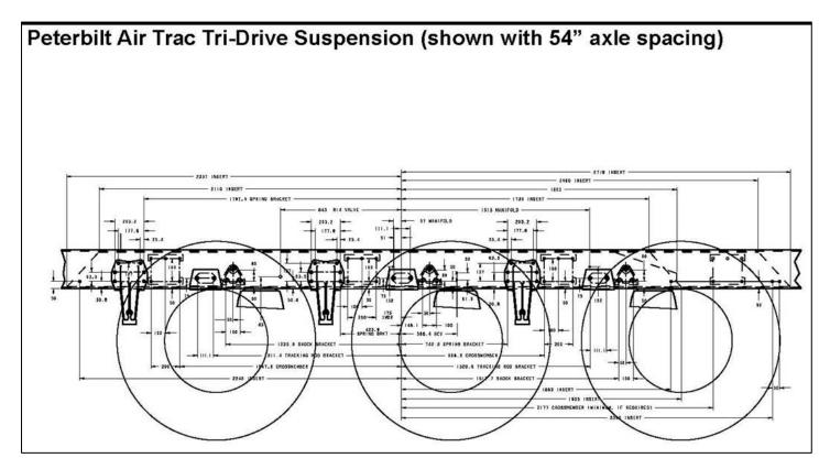
FIGURE 3-12. Peterbilt Air Trac Tri-Drive Frame Drilling (Dimensions In Millimeters)
