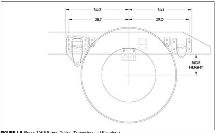
FIGURE 3-5. Reyco 79KB Frame Drilling (Dimensions In Millimeters)
