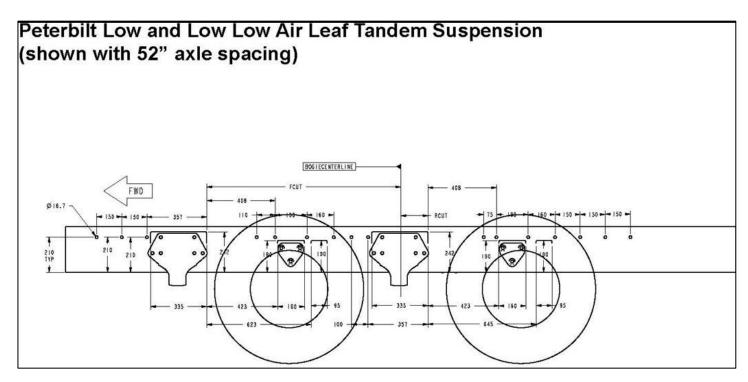
FIGURE 3-13. Peterbilt Low and Low-Low Air Leaf Tandem Frame Drilling (Dimensions In Millimeters)
