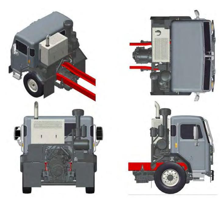
**FIGURE 3-32.** Exhaust Transverse DPF/SCR for ISX12 EPA 2013 Only (ISX12 didn't convert to 2017 Exhaust) See figure 3-1 for 2017 exhaust views showing all other engine configurations.
