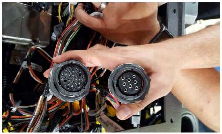
FIGURE 6-4. Body Builder Connections in Cab
