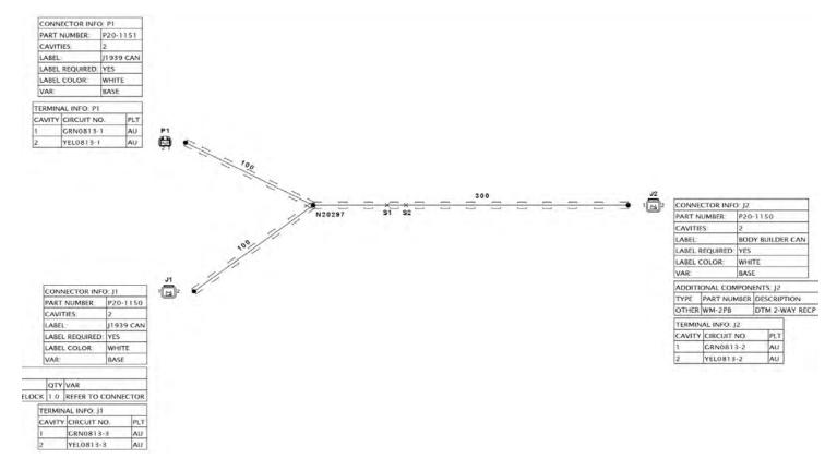
FIGURE 6-12. Harness S92-6160 Body Builder Connectors
