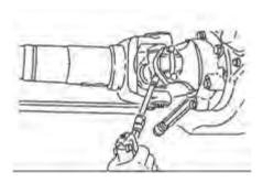
The slip joints and universal joints of the drive shaft should be lubricated according to Preventive Maintenance Schedule on page 5-12.
