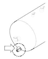
To eject moisture from the air system tanks, pull the line that is connected to the moisture ejection valve. Continue pulling until the air comes out free of water.
