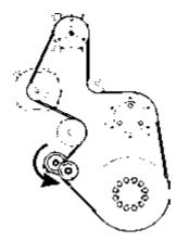
**Cummins Belt Routing**
