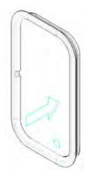
Press and slide the glass into the aft portion of the seal to seat it.
