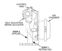
Brake Chamber Stroke
