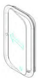
When the forward edge of the glass reaches the forward inside edge of the seal, the glass should pivot outboard into the remaining seal (see arrow in next illustration).
