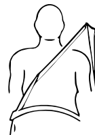
Figure 7: Seat Belt Twisted
