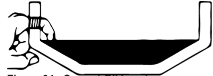
Figure 64: Correct Oil Level
