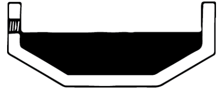
Figure 64: Correct Oil Level
