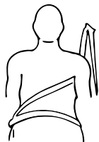
Figure 7: Seat Belt Twisted
