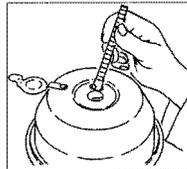
5. Assemble the release stud washer and nut on the release stud.
