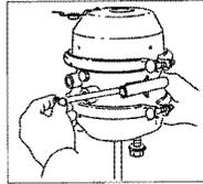
4. Insert the release stud through the opening in the spring chamber where the cap was removed. Insert it into the pressure plate. Turn the release stud 1/4 turn clockwise in the pressure plate. This secures the cross pin into the cross pin area of the pressure plate and locks it into the manual release position.
