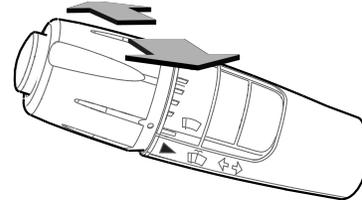
2. To return to previous beam, pull the **Turn Signal** lever towards the steering wheel again.
