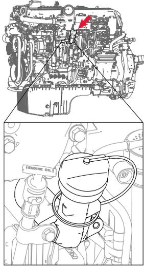
1. Top up with oil, if necessary, via the filler opening. Use the correct grade in the correct quantity. For oil replacement, please see engine Operator's Manual included with this chassis.
