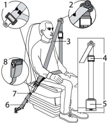
1. Web cut or frayed or extremely worn at latch area
