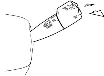
When in the Manual mode, the transmission gears can be manually selected by pushing or pulling on the lever. Pushing the lever forward will down shift. Pushing and holding the lever forward will engage the LOW gear range. Pulling the lever towards the driver will upshift the transmission.
