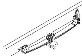
Each standard spring anchor pin has a grease fitting. Pressure lubricate spring pins as specified. At regular intervals, the spring leaves may be lubricated with a rust-inhibiting oil applied with a spray gun or brush. Depending on your suspension, lubricate all spring pins until grease flows out of both ends of the bushing. Look for signs of rust or water in the flushed grease. If a pin will not accept grease, it should be removed, cleaned, and inspected.
