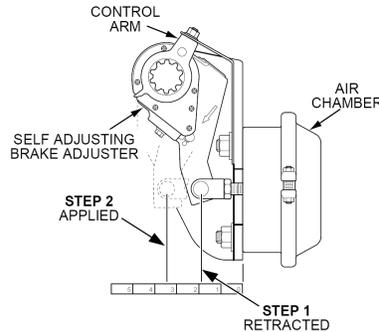
1. Retracted position, no brake pedal applied
