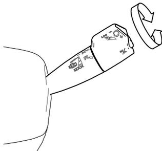
Transmission mode is selected by rotating the lever outer knob. There is a position for Drive (**D**), Neutral (**N**), and Reverse (**R**). The Digital Display will indicate the corresponding mode. See [Drive, Neutral, and Reverse Indicator](#).
