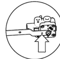
8. Torque the mounting fasteners to 55-75 lb-in. (6.2-8.5 N·m).
