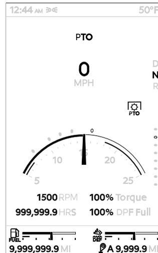
This truck may be equipped with Power Take-Off (PTO). PTO operation is enabled by using the dash mounted PTO switch in conjunction with the Cruise Control controls.
