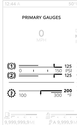
A gauge view presents the standard and optional virtual gauges monitoring your truck systems. Two single or two compound gauges can be shown per view. Gauges not shown in the first gauge view are shown in additional gauge views until all monitored systems are represented:
