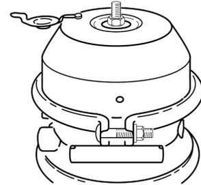
6. With a wrench, turn the release stud assembly nut until the compression spring is 90-95 percent caged. While doing this, ensure the push rod (adapter push rod or service push rod) is retracting. **DO NOT** over-torque the release stud assembly. (S-Cam-type maximum: 50 lb-ft (68 N·m), Wedge-type maximum: 30 lb-ft (41 N·m)). The spring brake is now mechanically released.
