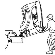
2. Place one or both hands at top of hood front, and tilt hood forward by pulling hood. Keep both feet on the ground for stability.
