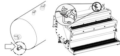
1. Turn the moisture ejection valve, or pull on the optional pull cord, until moisture comes out the valve.
