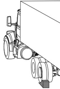
3. Drain water from the air reservoirs. Open the reservoir drains just enough to drain the moisture. Don't deplete the entire air supply. Be sure to close the drains before leaving the vehicle.
