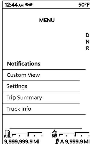
The menu allows the operator to view active warnings, truck performance, activate and customize vehicle features, and access trip information. The menu can only be accessed when the parking brake is set.<sup>8</sup> Use the **Scroll** to choose the menu
