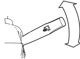
Moving the lever clockwise will engage the engine brake. Increase the amount of engine brake by moving the lever further clockwise. Each position has a corresponding level of engine brake.
