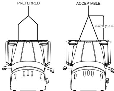
Use a double chain or cable setup that distributes the load equally to both hitches (see either example in Recovery Rigging Options illustration):
