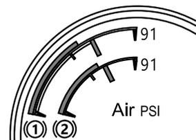
3. Build up air pressure in the system until the system cutout setpoint or until 120 psi (827 kPa) is reached.
