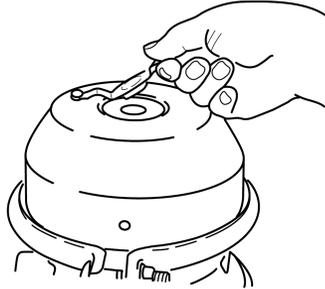
2. Remove the release stud assembly from the side pocket, and remove the release nut and washer from the release stud.
