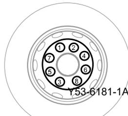
Proper wheel torque can best be obtained on level ground. Install lug nuts and finger-tighten in the numerical sequence as shown below. This procedure will ensure that the wheel is drawn evenly against the hub. Contact an authorized dealer for information on the proper installation procedure for the wheels on your truck. This is a job you may not be able to do yourself. You need the right torquing equipment to do it.
