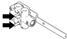
6. Rotate the valve either clockwise or counterclockwise until air pressure in the air springs provides the ride height specified for that suspension. Measure the ride height from the bottom of the frame rail to the approximate centerline of the rearmost drive axle hub:
