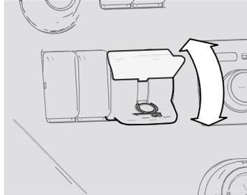
Press the lever down to engage the Trailer Hand Brake. Push the lever back up to release the Trailer Hand Brake.
