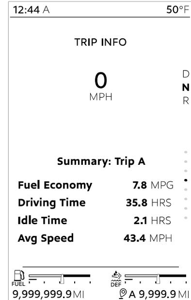
Presents information concerning truck use during the current trip. These details will be collected until the trip is reset, or the max trip distance (99,999.9 miles for main, 9,999.9 for sub-trips) is reached. For
