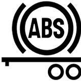
1. It illuminates during the power-on self test when the ignition is turned ON. It turns off after a few seconds if no system problems are detected. The bulb self-test is performed whenever the ignition is turned ON, regardless of whether
