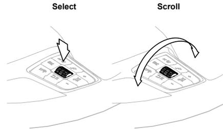
For example, vehicle time can be set using the Scroll Wheel.
