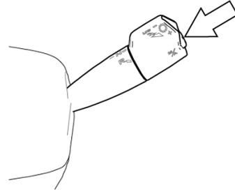
This button will put the transmission into manual mode. Manual mode will allow the operator to select the gear (See Upshifting and Downshifting).
