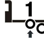
Turn switch on to lower Single or Forward Pusher Axle.
