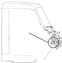
3. Locate the filter cover labeled "OPEN" with an arrow pointing towards the rear of the vehicle. Slide the filter cover towards the rear of the vehicle, until you are able to remove the cover.
