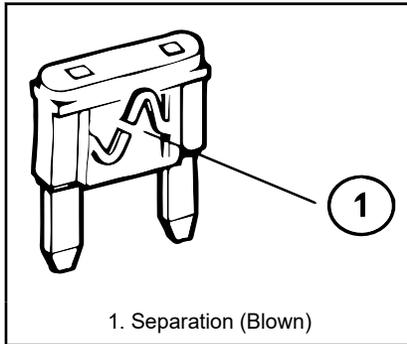
3. If it is blown, replace it with a fuse of the same rating. If a fuse of the same rating is not available, a fuse of a lower rating may be temporarily substituted. You can also use a fuse from a circuit you
