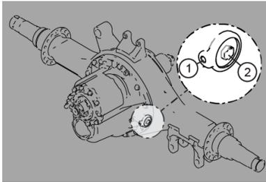
1. Remove the air line and firmly cap the air line from the vehicle. (2)
