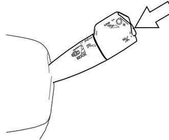
This button will put the transmission into manual mode. Manual mode will allow the operator to select the gear. See [Up or Down Shifting](#) on page 151.
