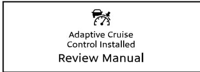
This indication at vehicle start means it is equipped with Adaptive Cruise Control (ACC) and Collision Mitigation. These features work together to improve driver safety and enhance the driving experience. When Cruise Control is active, ACC will accelerate and slow the truck to maintain a chosen distance from a detected forward vehicle. Collision Mitigation will attempt to prevent a forward collision when advancing at speeds greater than 15 mph (24 kph). Please review the ACC section of this
