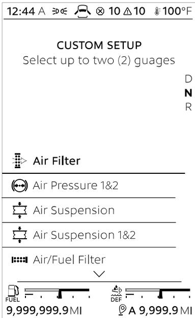
Vehicles with this option provide a view which can contain up to four operator-selected gauges. If the custom view has
