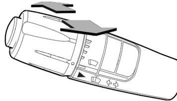
2. The lever will automatically return when the lever is released. The blue indicator light in the instrument panel will momentarily turn on and the high beams will flash. The high beams will not remain on if the lever is still pressed.
