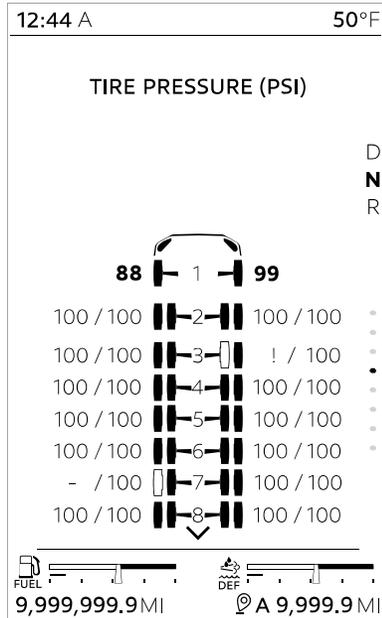
The Tire Pressure Monitoring System (TPMS) is an optional feature combining tire data with the chassis axle layout, displayed graphically. The TPMS can be
