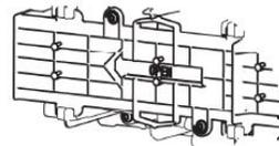
4. Remove and inspect the filter, referring to the maintenance interval schedule.
