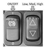
By pressing the left switch, the driver can turn the regen braking on and off. By pressing the right switch, the driver can toggle through three available levels.
