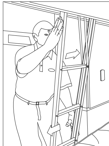
Figure 4: Hand Positions to Fold the Ladder
