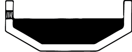
Figure 68: Correct Oil Level
