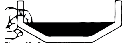
Figure 68: Correct Oil Level
