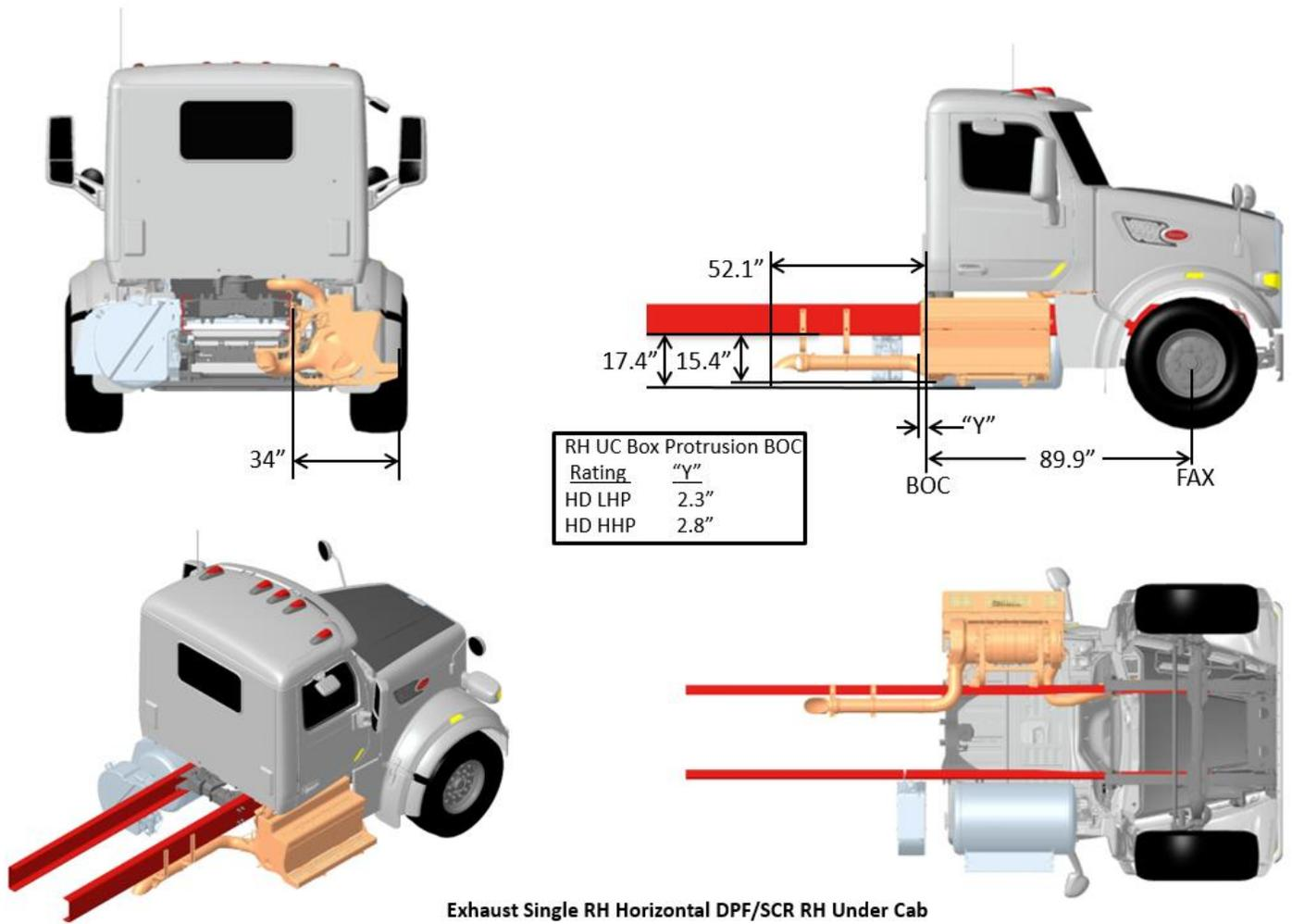
**FIGURE 3-65.** Exhaust Single RH Horizontal DPF/SCR RH Under Cab
