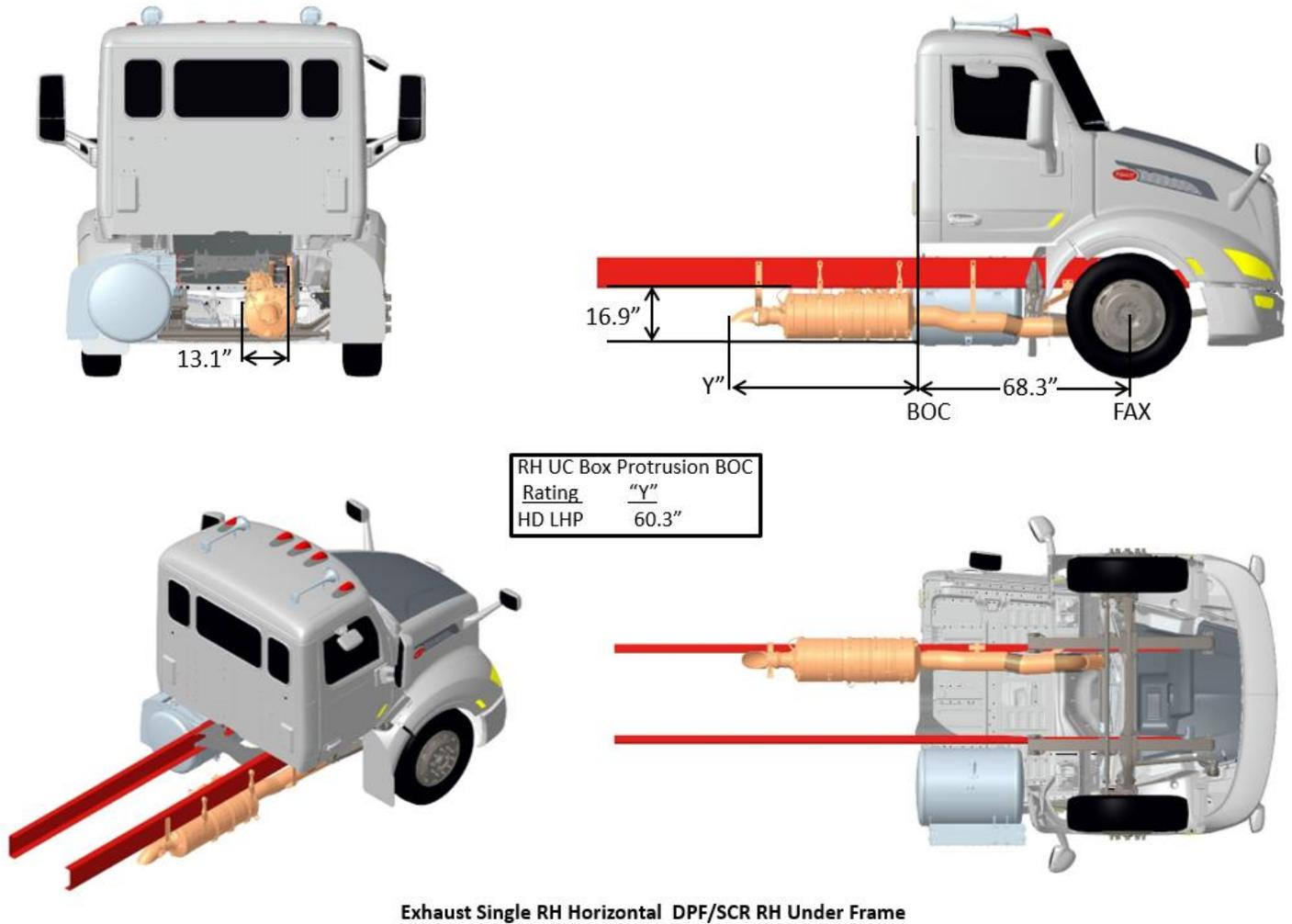
FIGURE 3-73. Exhaust Single RH Horizontal DPF/SCR RH Under Frame
