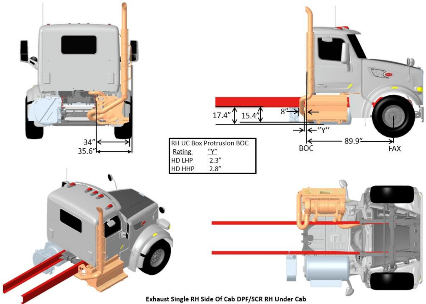
FIGURE 3-64. Exhaust Single RH Side of Cab DPF/SCR RH Under Cab
