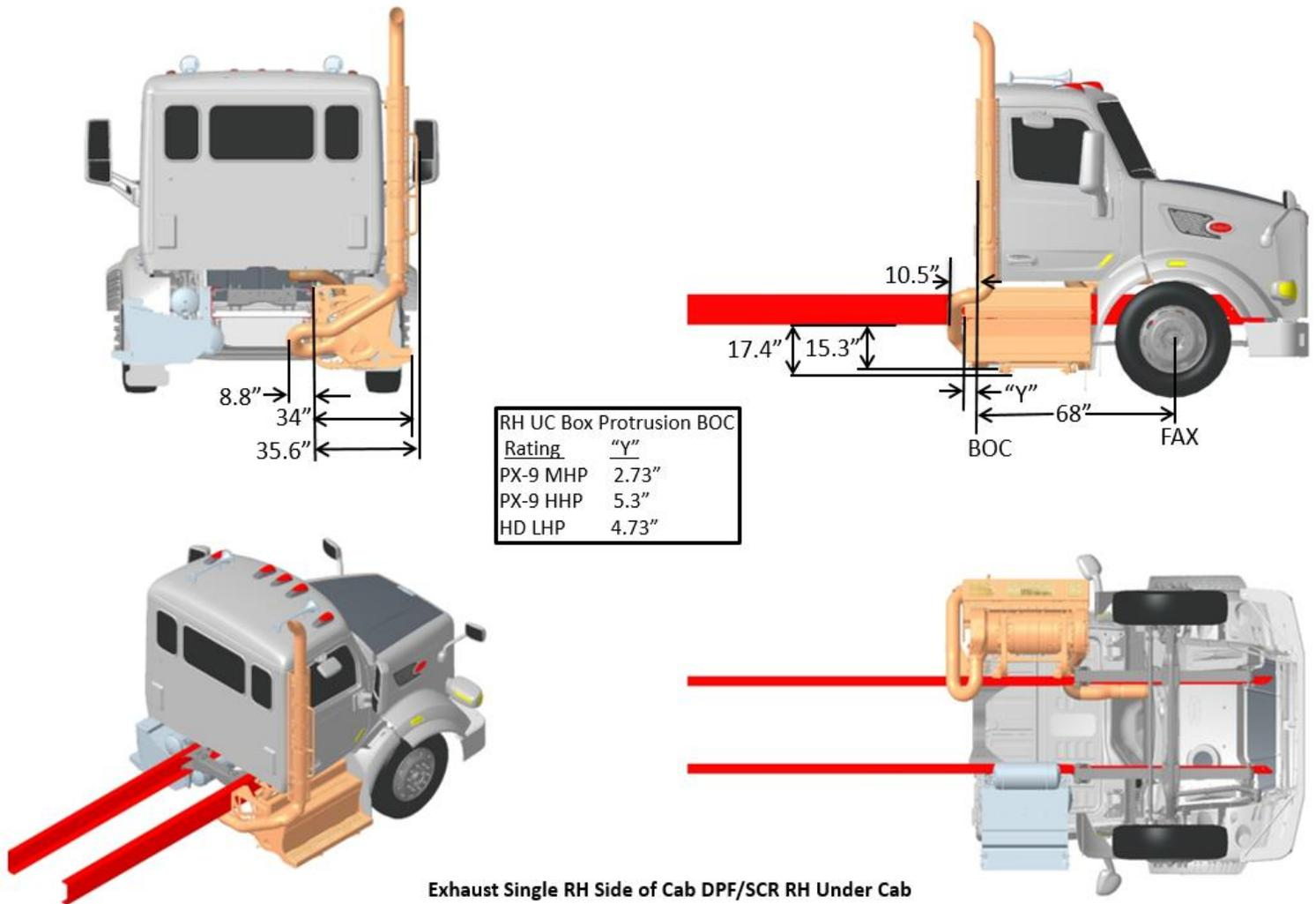
FIGURE 3-43. Exhaust Single RH Side of Cab DPF/SCR RH Under Cab
