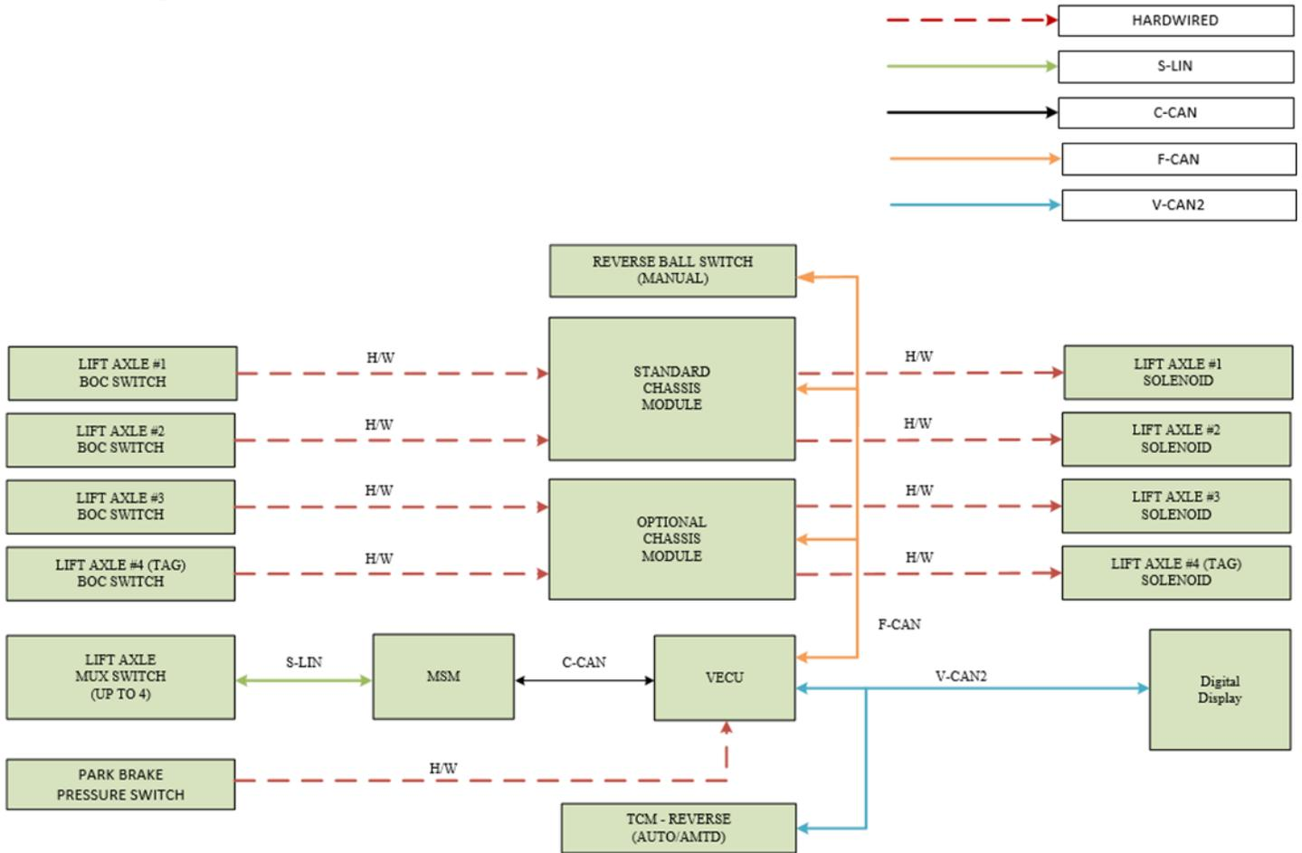
**Truck Lift Axle Logic**
