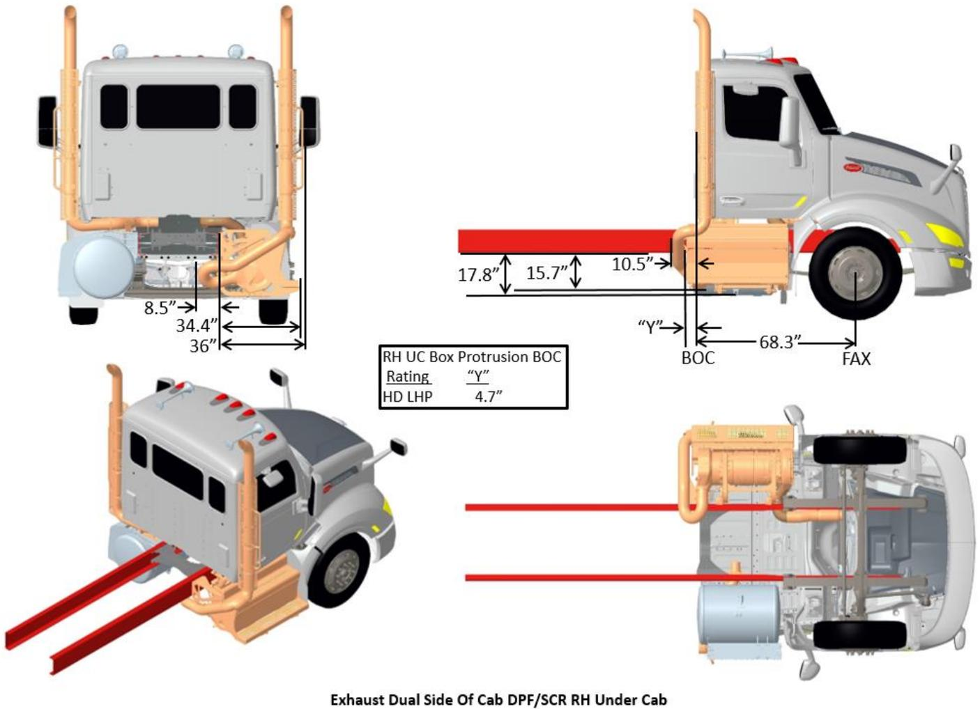
FIGURE 3-74. Exhaust Dual SOC DPF/SCR RH Under Cab
