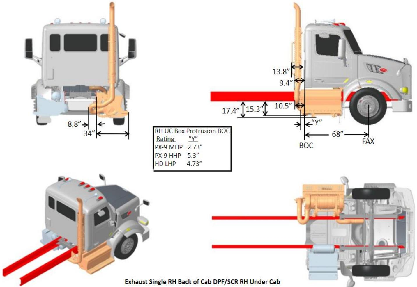
Exhaust Single RH Back of Cab DPF/SCR RH Under Cab
