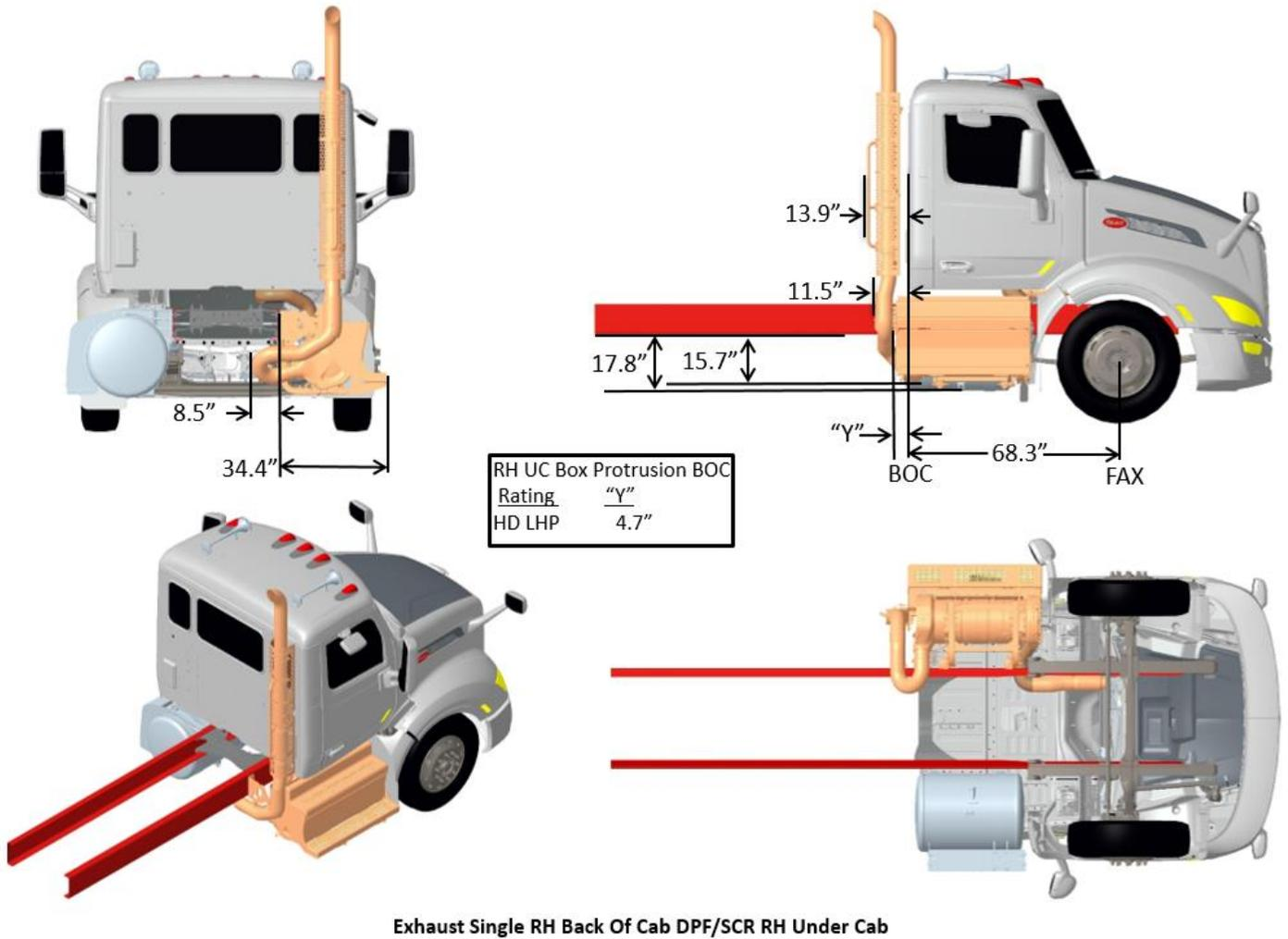
FIGURE 3-70. Exhaust Single RH Back of Cab DPF/SCR RH Under Cab
