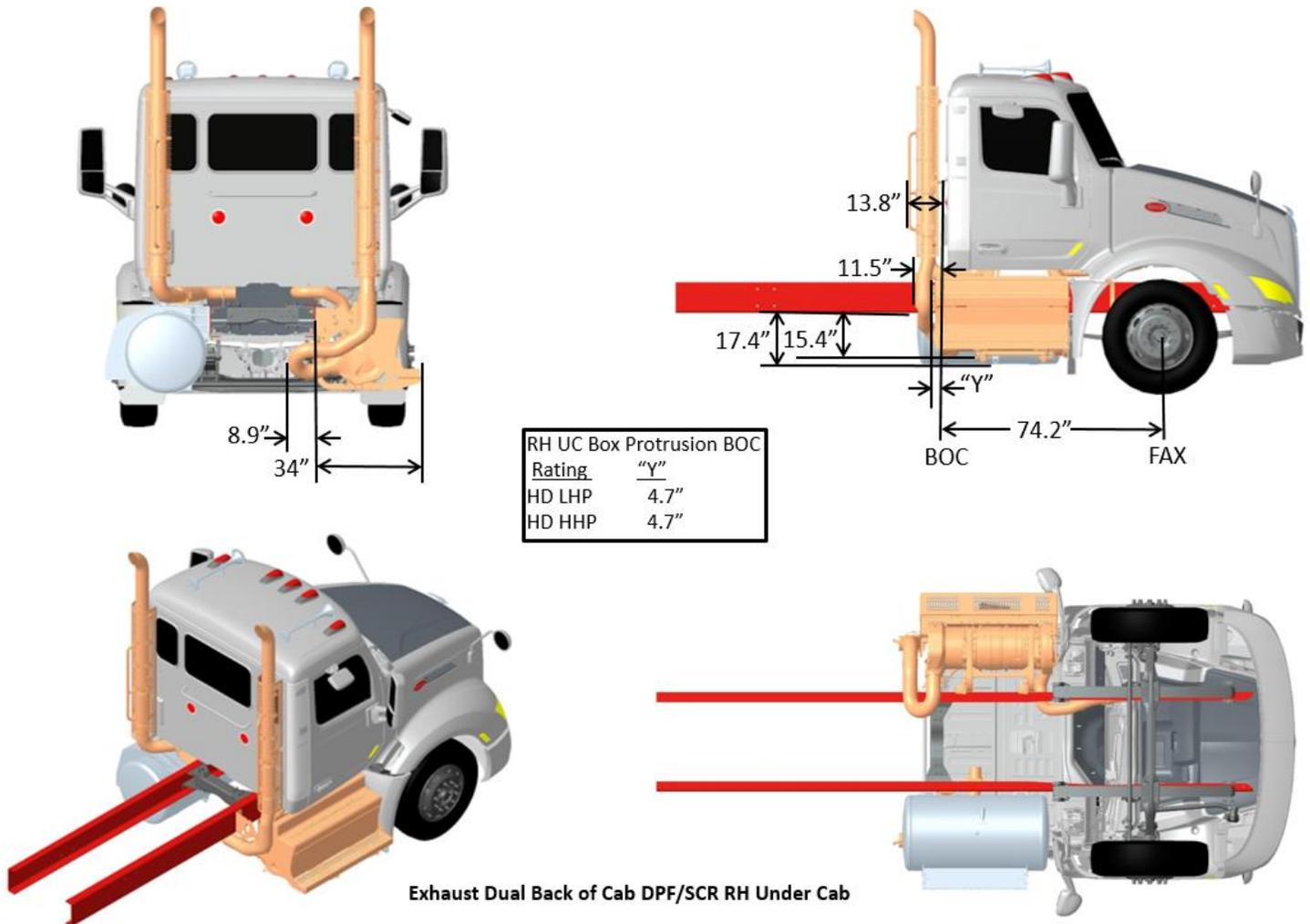
FIGURE 3-82. Exhaust Dual Back of Cab RH DPF/SCR RH Under Cab
