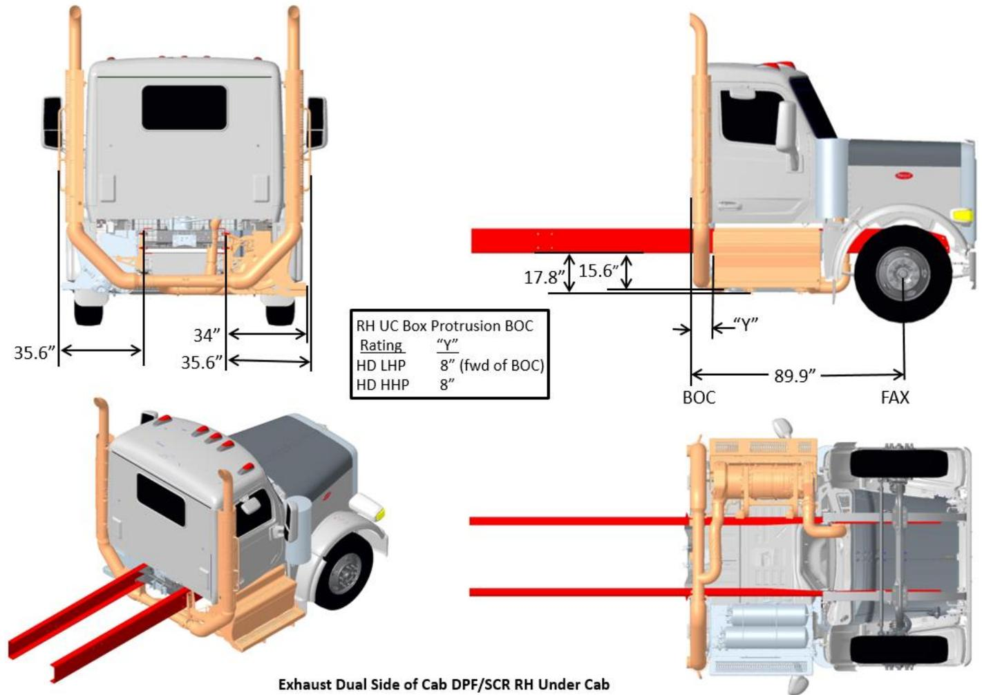
**FIGURE 3-34.** Exhaust Dual Side of Cab DPF/SCR RH Under Cab (functioning)
