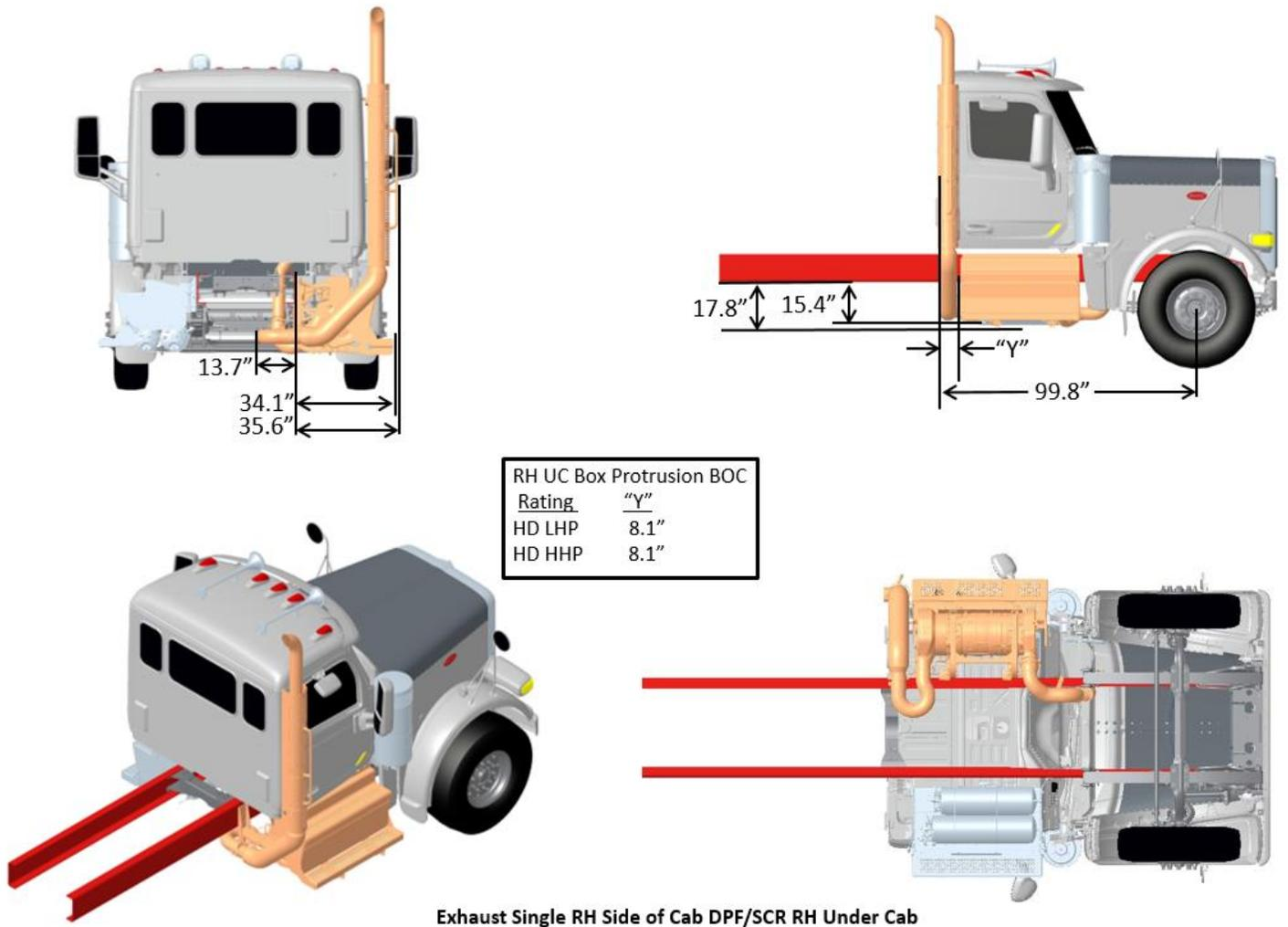
**FIGURE 3-37.** Exhaust Single RH Side of Cab DPF/SCR RH Under Cab
