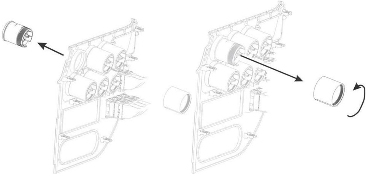
Optional gauges may be installed and connected to the Digital Display via a jumper harness.
