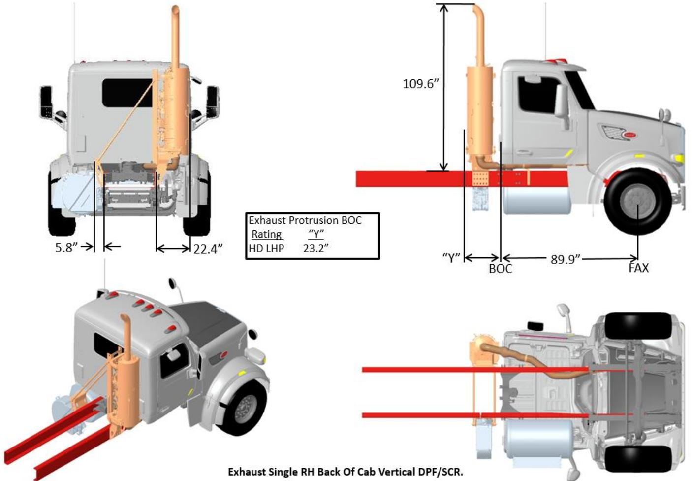
FIGURE 3-69. Exhaust Single RH BOC Vertical DPF/SCR
