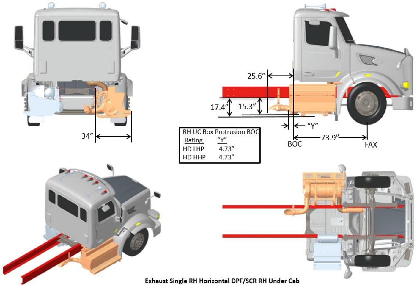
**FIGURE 3-58.** Exhaust Single RH Horizontal DPF/SCR RH Under Cab
