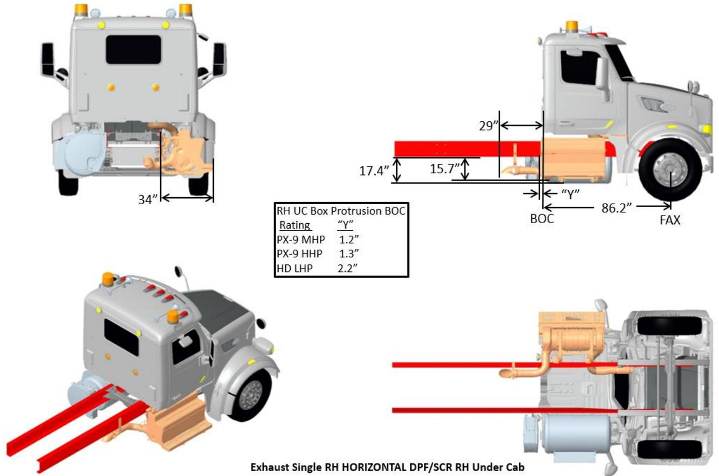
**FIGURE 3-51.** Exhaust Single RH Horizontal DPF/SCR RH Under Cab
