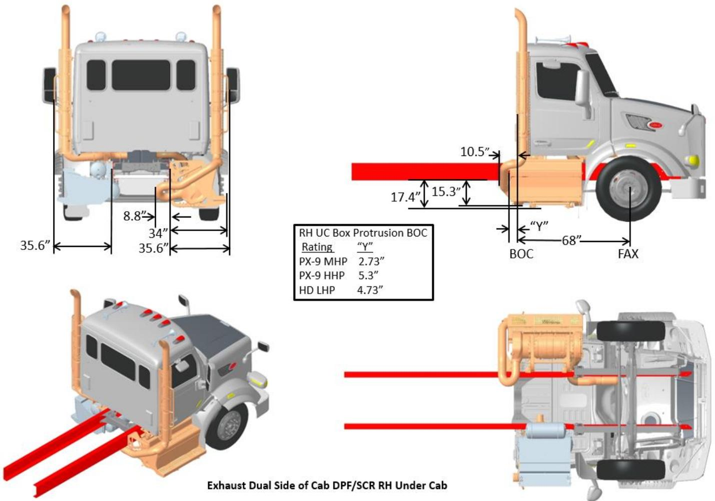
**FIGURE 3-46.** Exhaust Dual SOC DPF/SCR RH Under Cab
