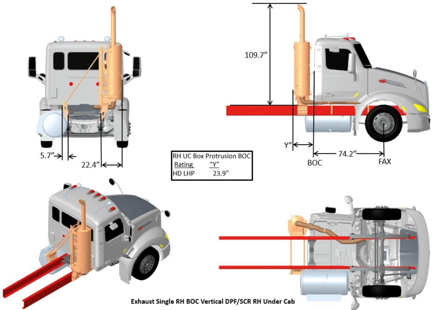
FIGURE 3-83. Exhaust Single RH BOC Vertical DPF/SCR
