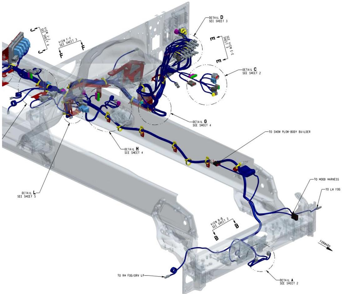
DETAIL VIEW OF ENGINE COMPARTMENT BODY CONNECTORS
