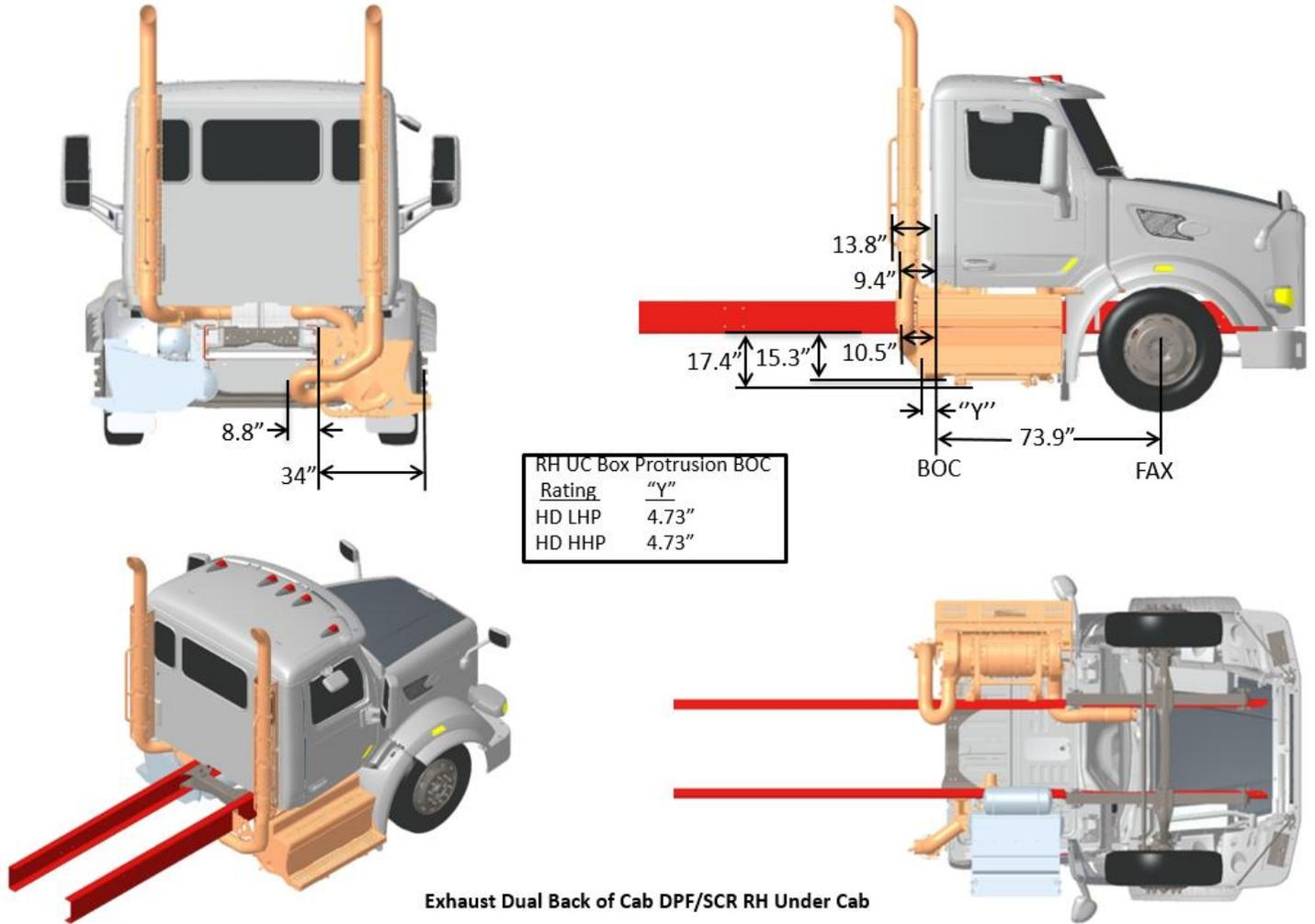
FIGURE 3-62. Exhaust Dual Back of Cab DPF/SCR RH Under Cab
