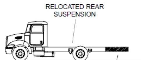
CUT FRAME AT REAR TO OBTAIN DESIRED CUTOFF
