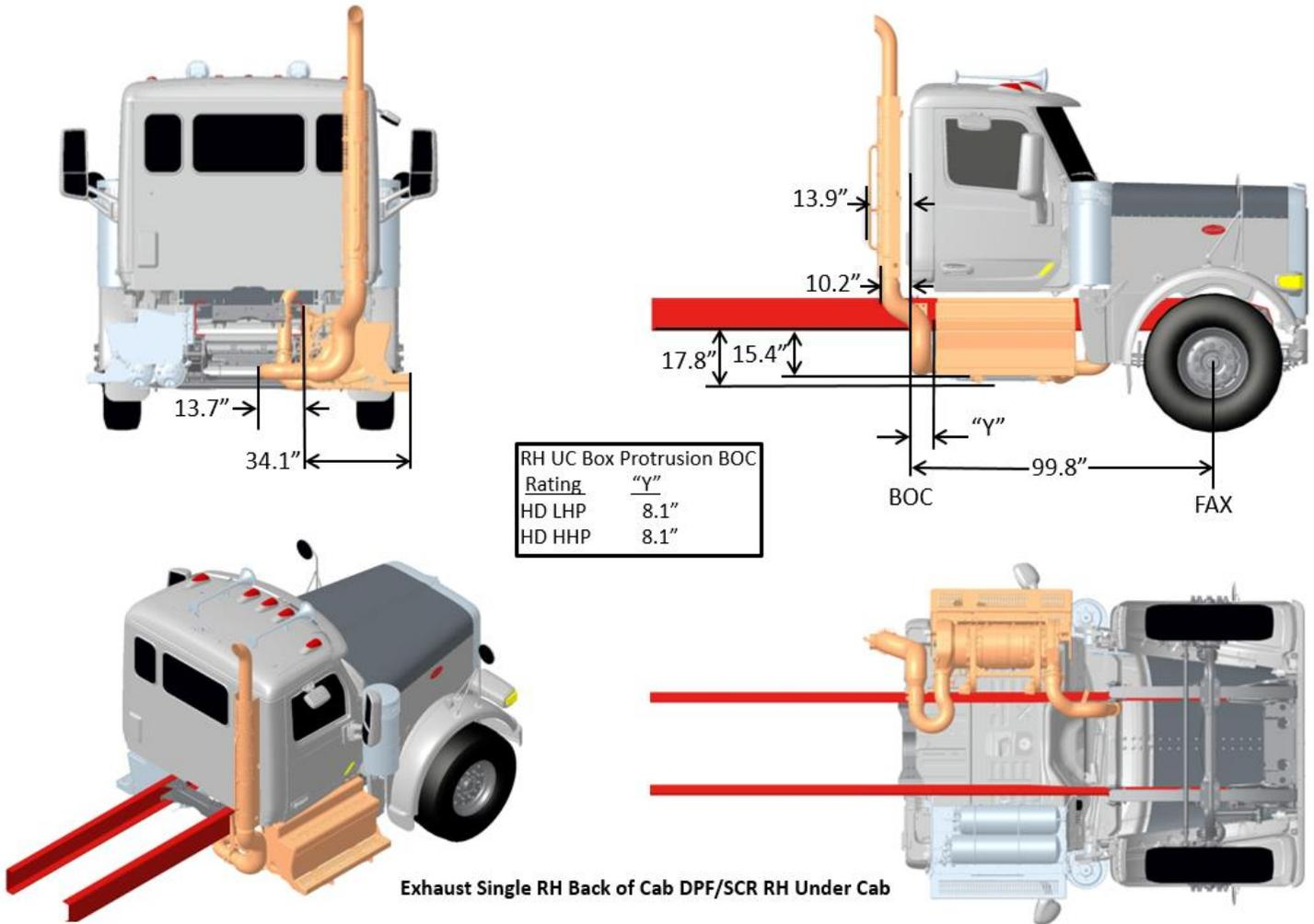
FIGURE 3-36. Exhaust Single RH Back of Cab DPF/SCR RH Under Cab
