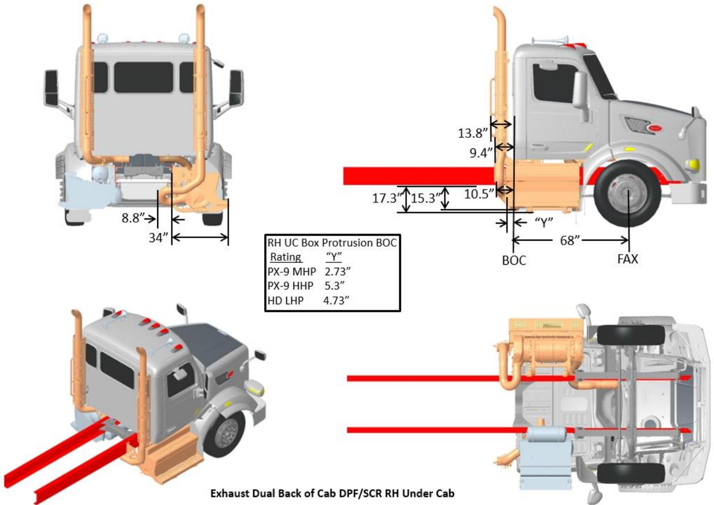
**FIGURE 3-47.** Exhaust Dual BOC DPF/SCR RH Under Cab
