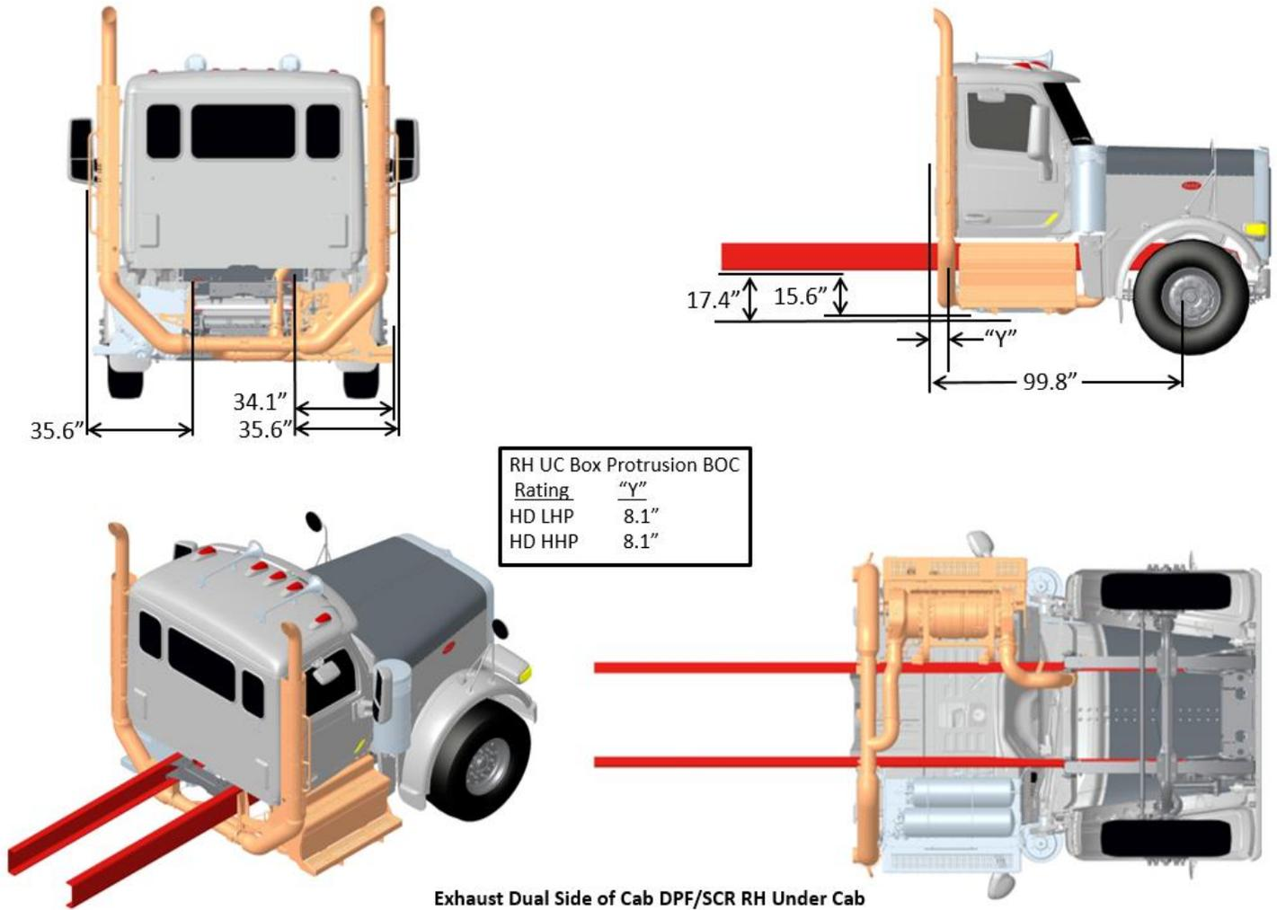
**FIGURE 3-40.** Exhaust Dual Side of Cab DPF/SCR RH Under Cab (functioning)
