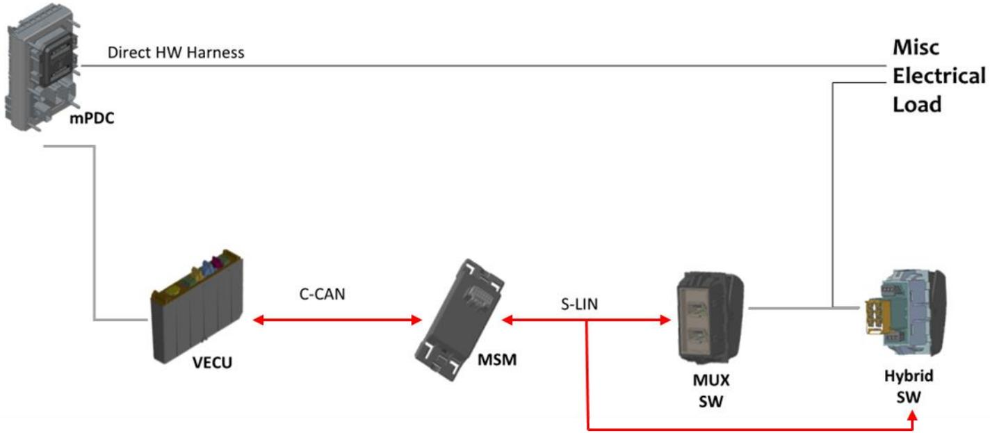
Multiplexing = shorter wire bundles, improved diagnostics, and greater driver feedback. Safety critical switches use hybrid switch with hardwire for redundancy. The switches are less expensive with fewer wires behind the dash and on the chassis. The switches are self-diagnosable to improve troubleshooting with DAVIE.
