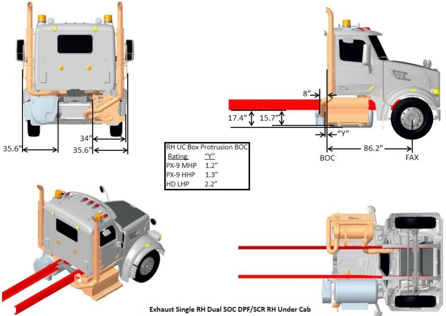
**FIGURE 3-53.** Exhaust Dual SOC DPF/SCR RH Under Cab
