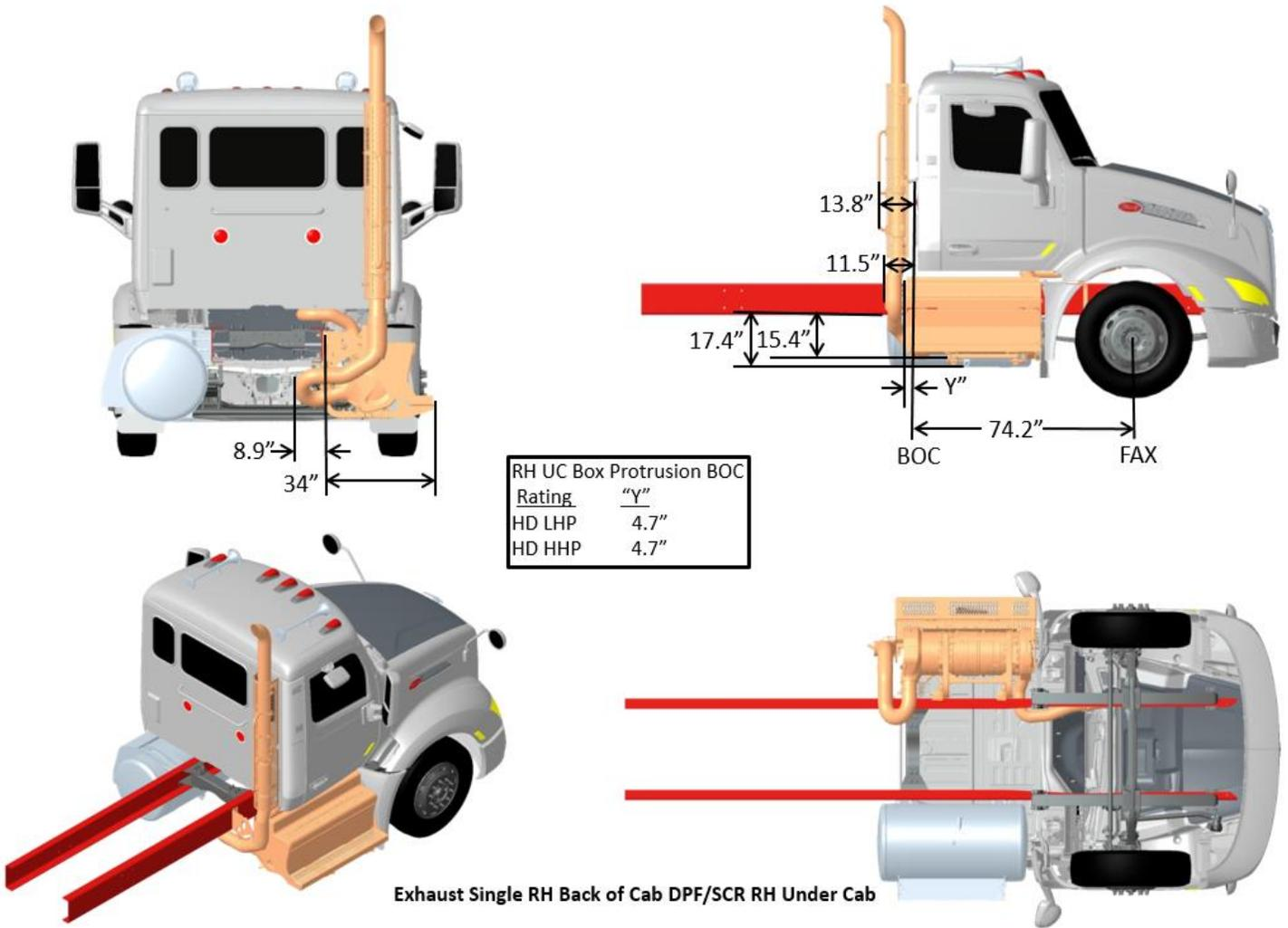
FIGURE 3-77. Exhaust Single RH Back of Cab DPF/SCR RH Under Cab
