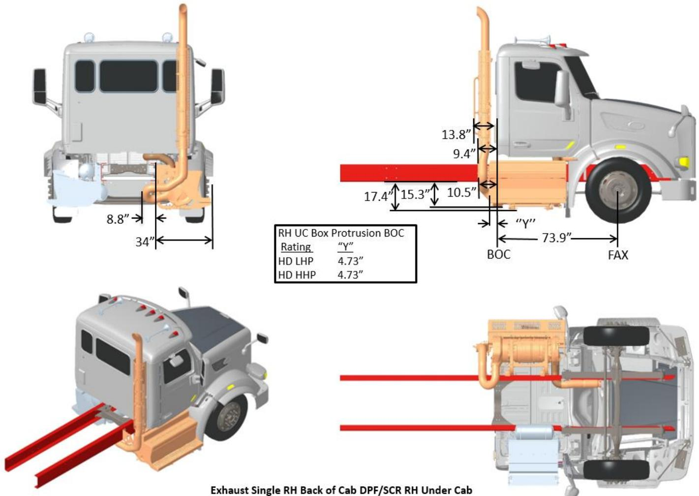
FIGURE 3-56. Exhaust Single RH Back of Cab DPF/SCR RH Under Cab
