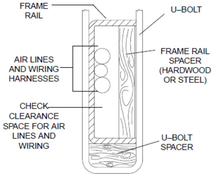
FIGURE 4-10. Clearance Space for Air Lines and Cables
