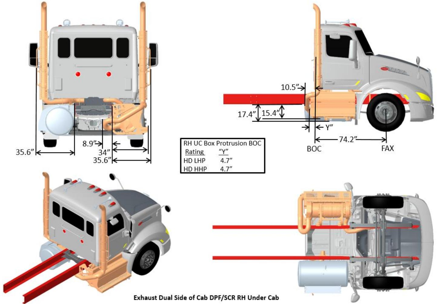
**FIGURE 3-81.** Exhaust Dual Side of Cab RH DPF/SCR RH Under Cab
