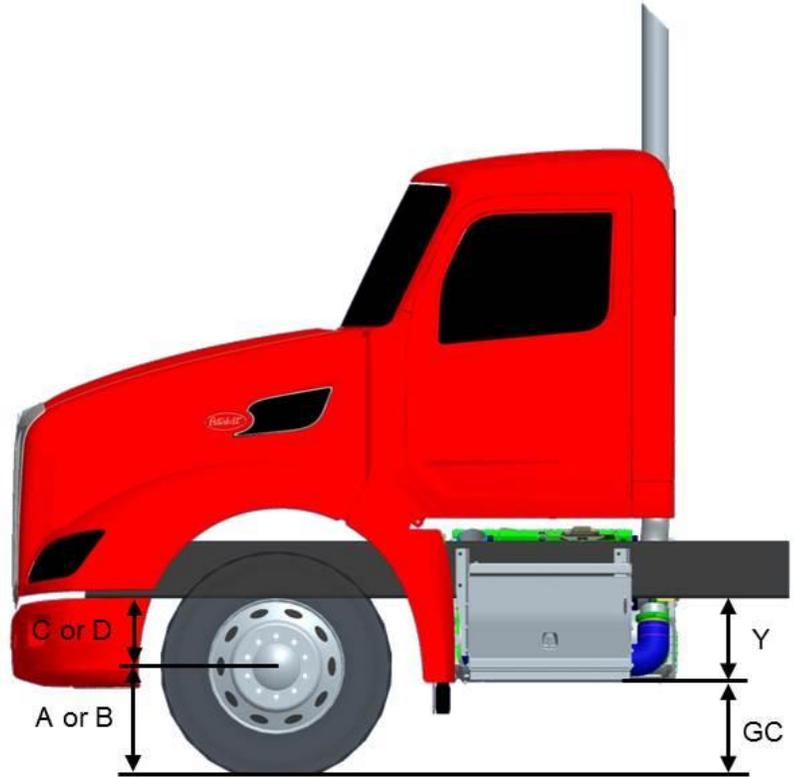
**FIGURE 3-26.** Ground Clearance Calculations
