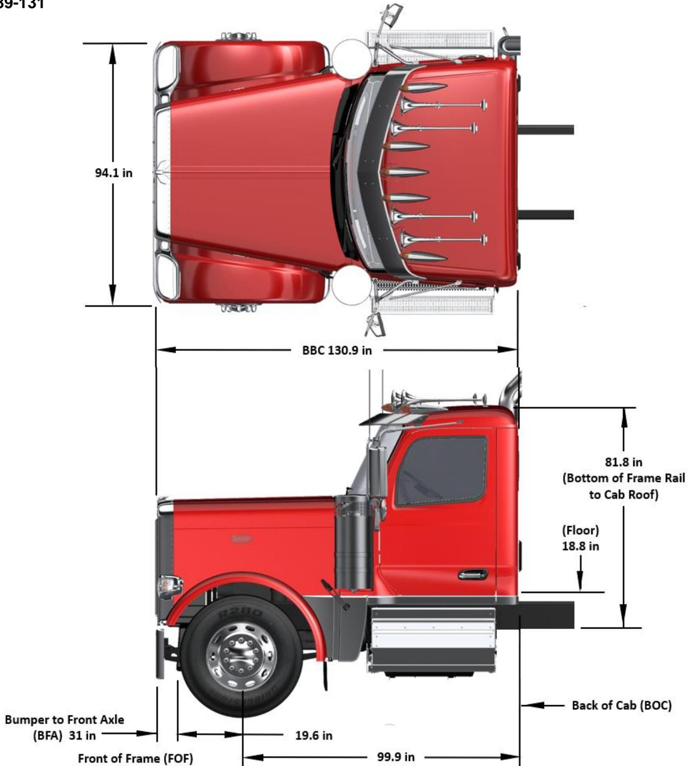
FIGURE 3-2. Model 589-131 Top & LH View – Overall Dimensions
