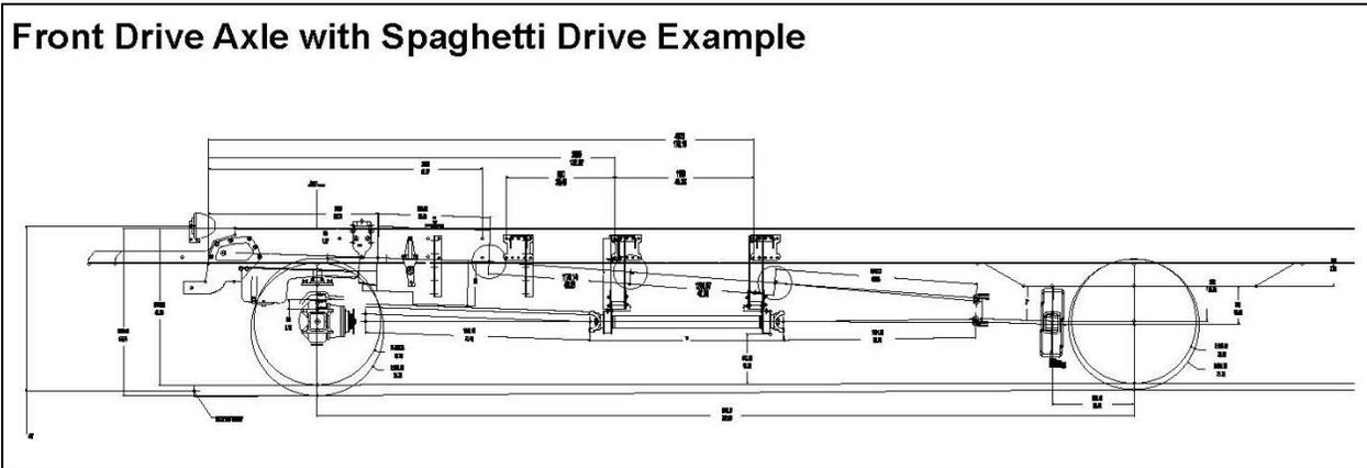
**FIGURE 3-13.** Front Drive Axle with Spaghetti Drive Example
