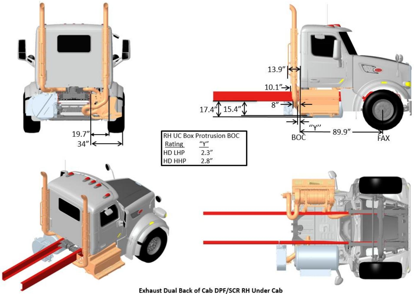
FIGURE 3-67. Exhaust Dual Back of Cab DPF/SCR RH Under Cab
