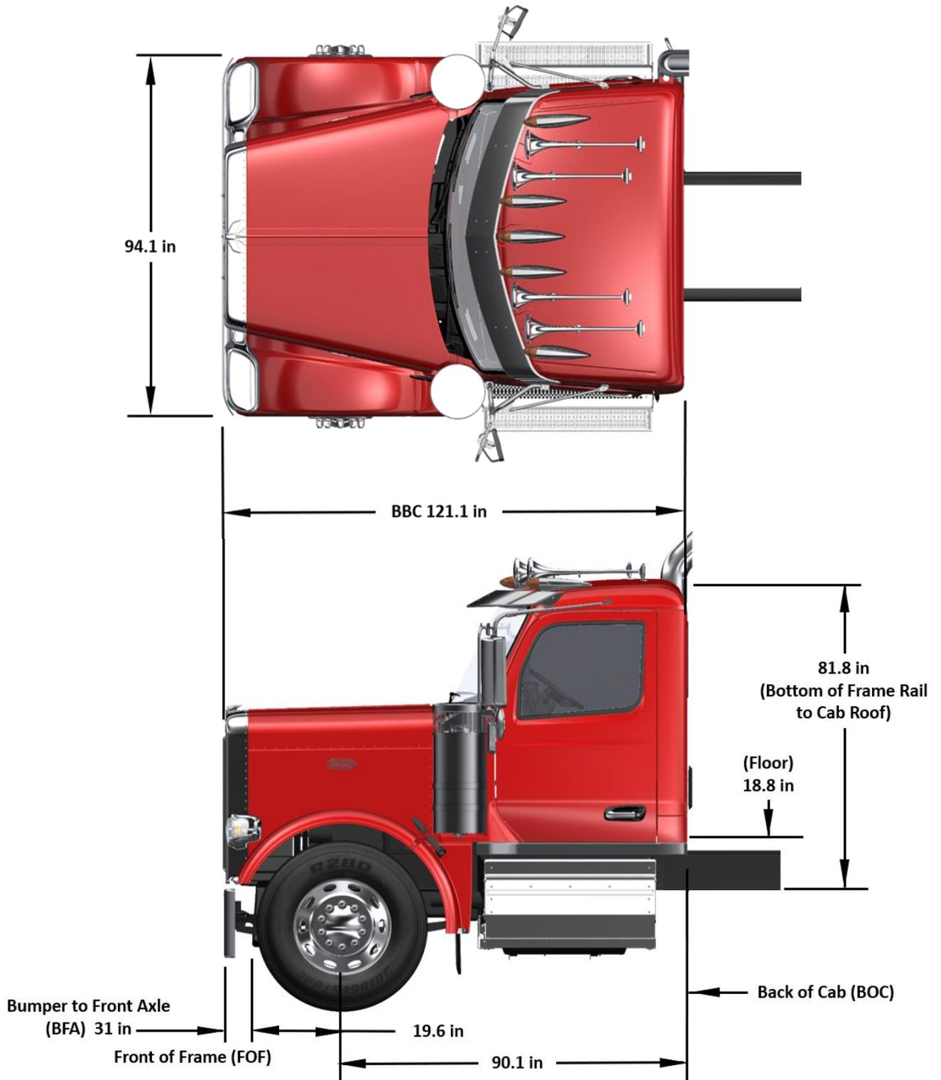
**FIGURE 3-1.** Model 589-121 Top & LH View – Overall Dimensions
