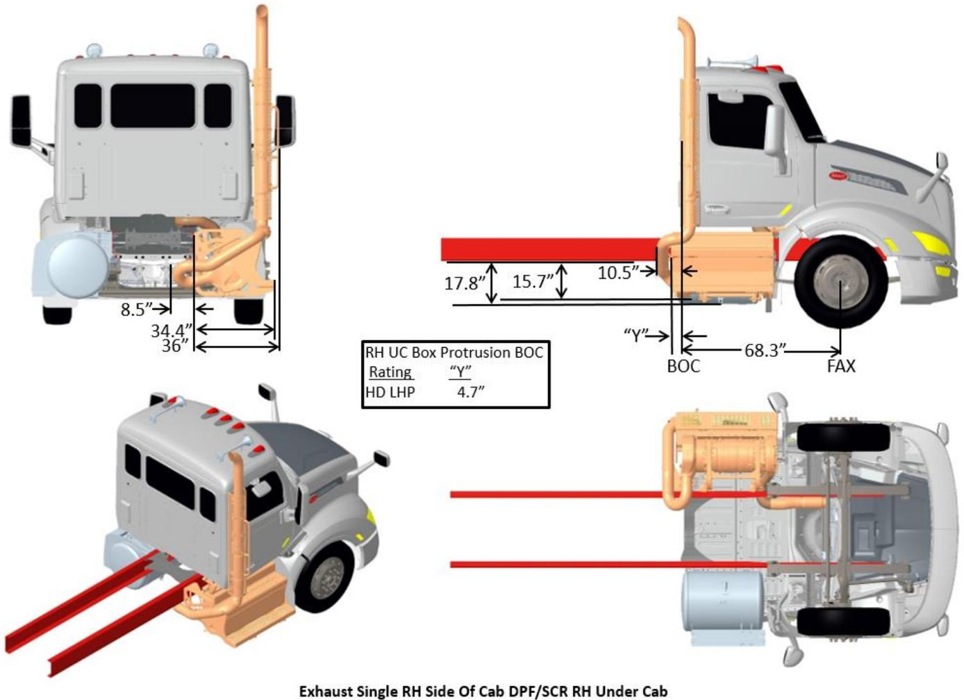
FIGURE 3-71. Exhaust Single RH Side of Cab DPF/SCR RH Under Cab
