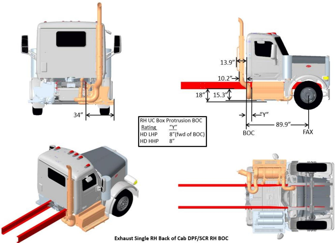
FIGURE 3-30. Exhaust Single RH Back of Cab DPF/SCR RH Under Cab
