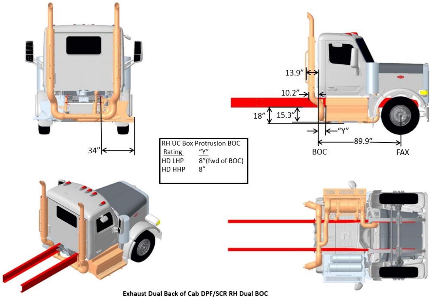
**FIGURE 3-35.** Exhaust Dual Back of Cab DPF/SCR RH Under Cab (functioning)
