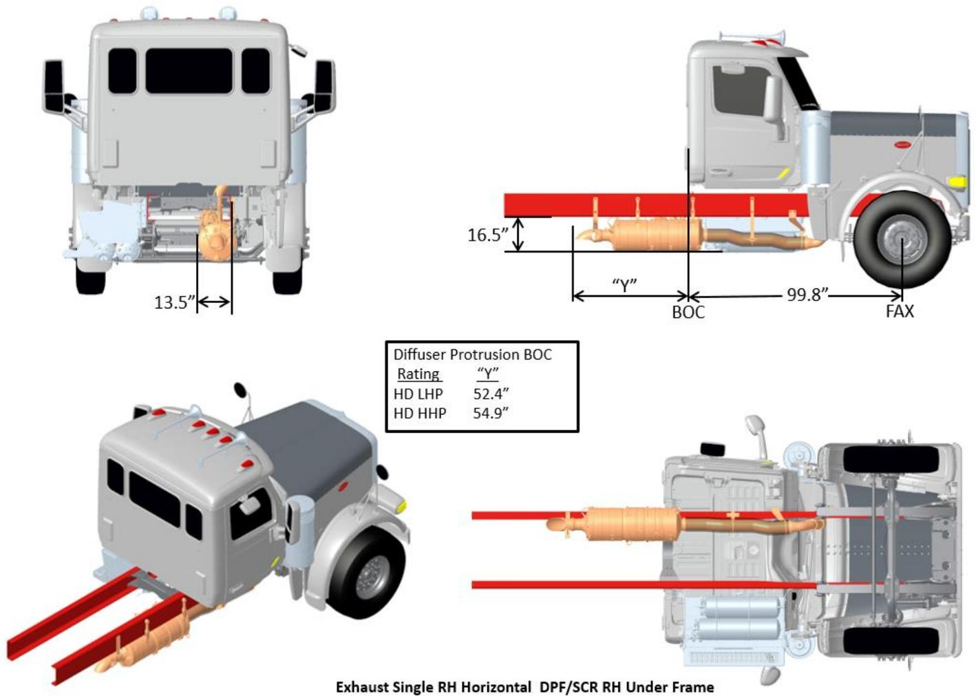
FIGURE 3-39. Exhaust Single RH Horizontal DPF/SCR Under Frame
