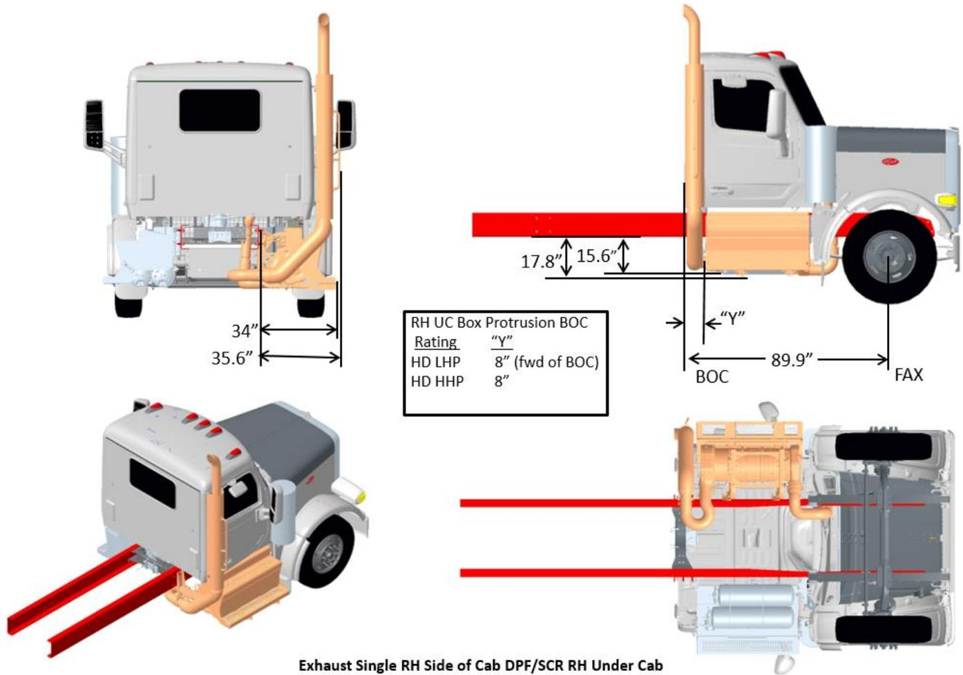
**FIGURE 3-31.** Exhaust Single RH Side of Cab DPF/SCR RH Under Cab
