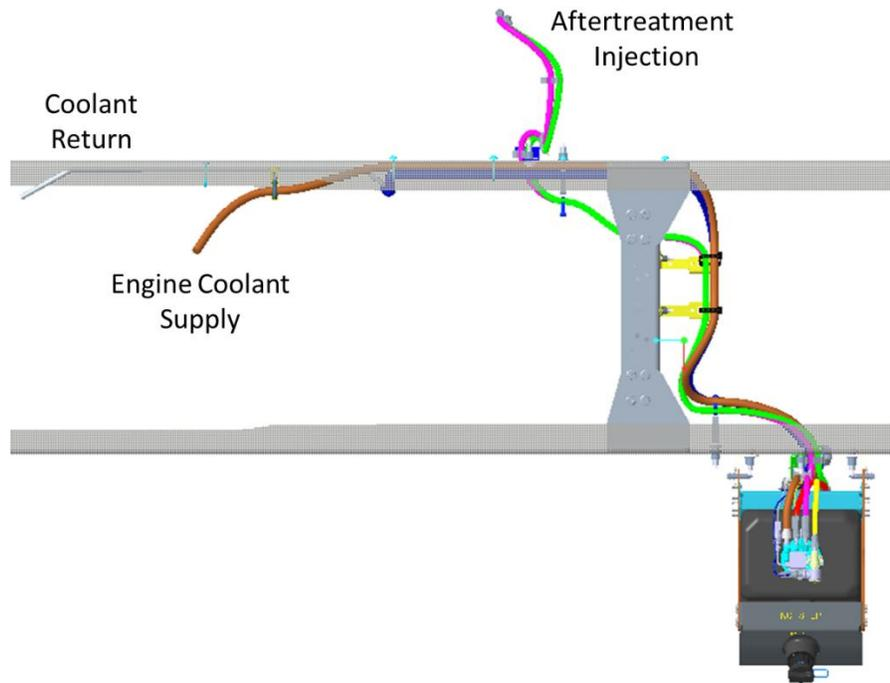
**FIGURE 9-3.** Routing for DEF and Coolant Lines
