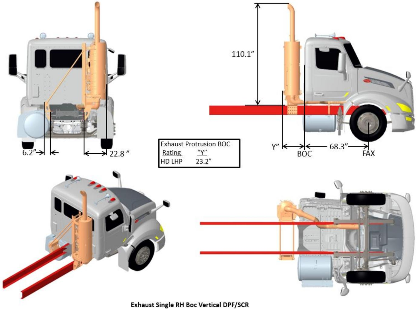
FIGURE 3-76. Exhaust Single RH Boc Vertical DPF/SCR
