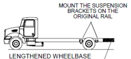
DO NOT MOUNT THE SUSPENSION BRACKET ON THE ADDED FRAME RAIL
