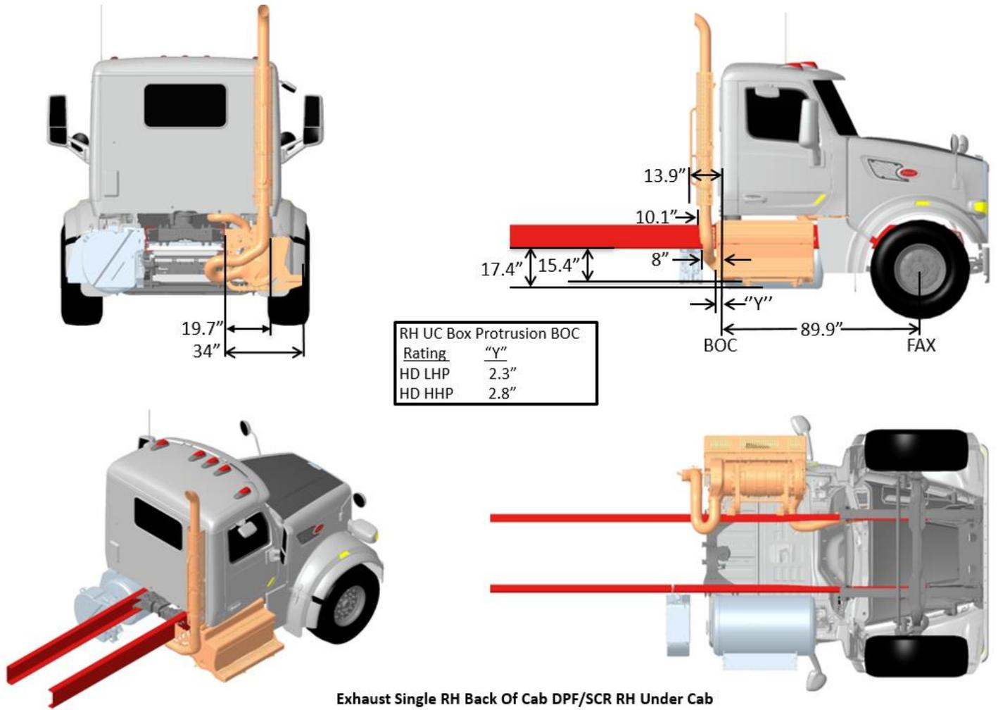
FIGURE 3-63. Exhaust Single RH Back of Cab DPF/SCR RH Under Cab
