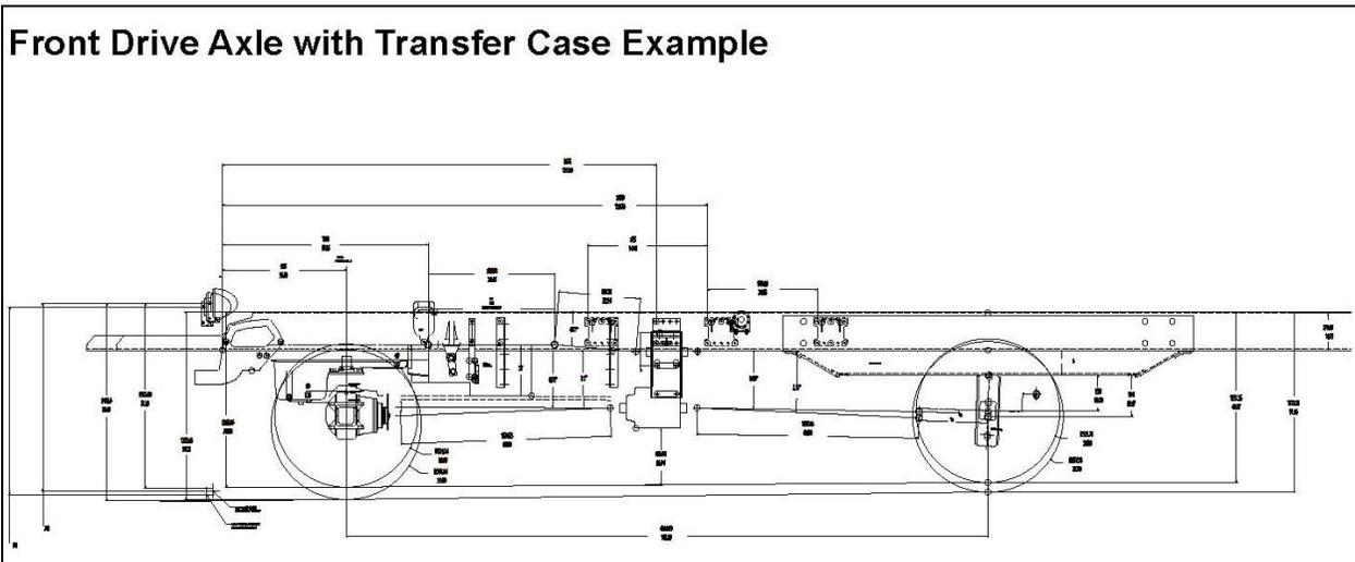
**FIGURE 3-14.** Front Drive Axle with Transfer Case Example
