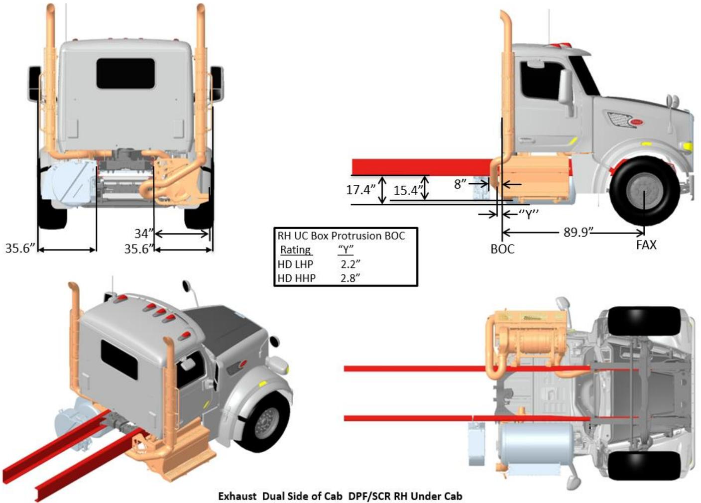
FIGURE 3-68. Exhaust Dual SOC DPF/SCR RH Under Cab
