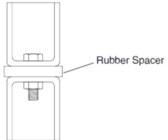
**FIGURE 4-5.** Mounting Brackets
