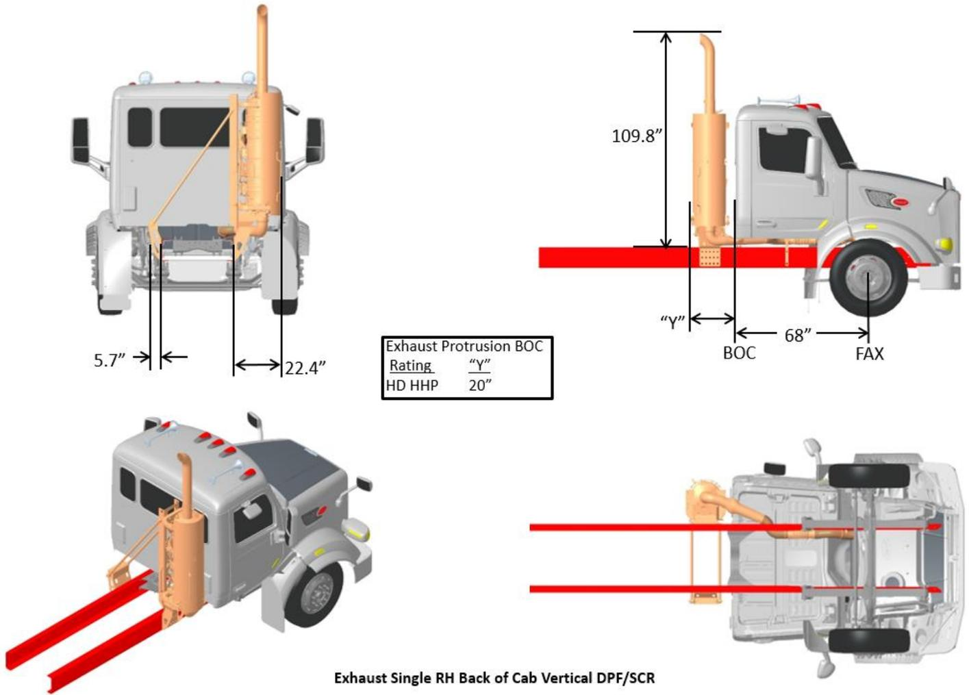
FIGURE 3-48. Exhaust Single RH BOC Vertical DPF/SCR
