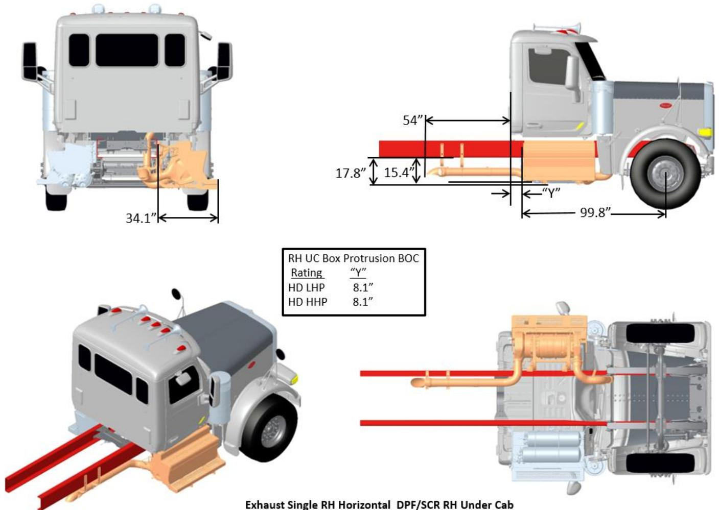
FIGURE 3-38. Exhaust Single RH Horizontal DPF/SCR RH Under Cab
