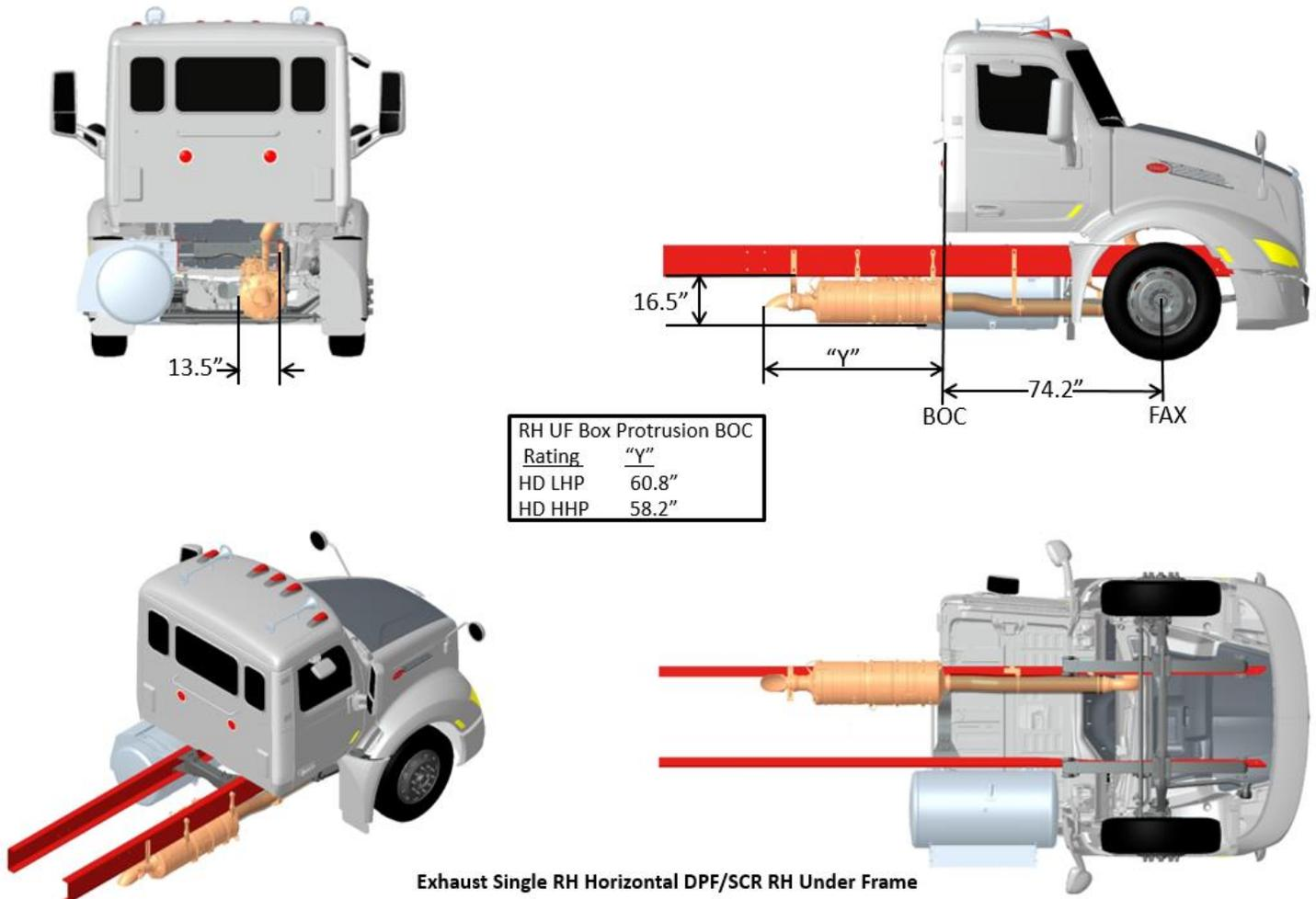
FIGURE 3-80. Exhaust Single RH Horizontal DPF/SCR RH Under Frame
