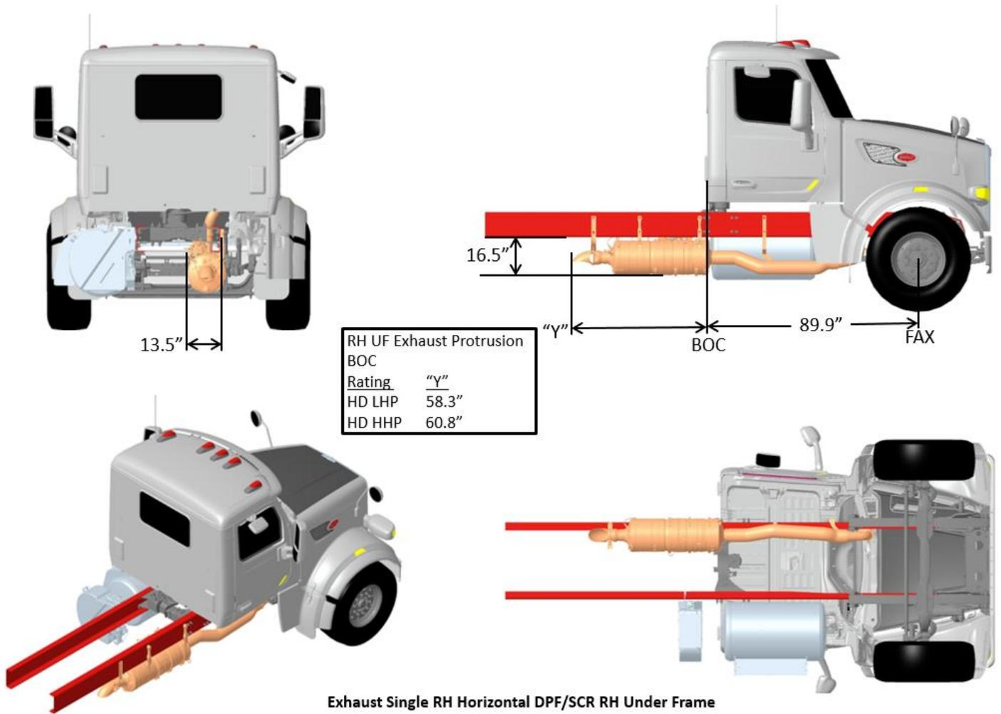
FIGURE 3-66. Exhaust Single RH Horizontal DPF/SCR RH Under Frame
