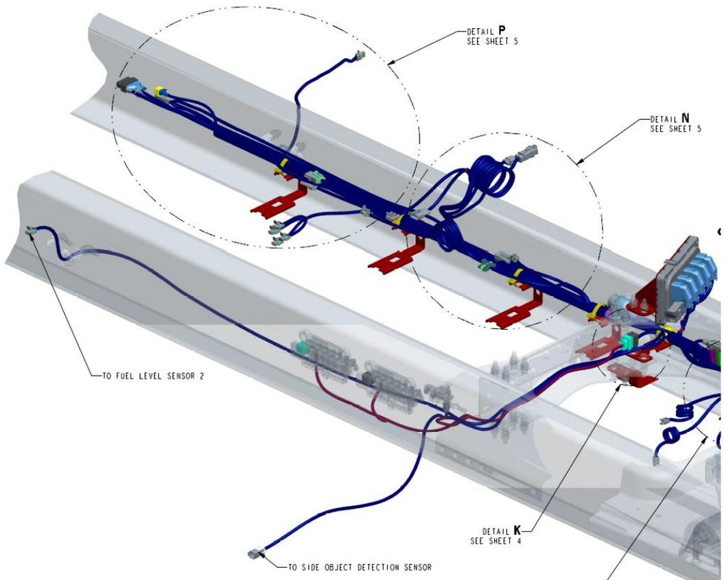
DETAIL VIEW OF BOC/BOS AND EOF BODY CONNECTORS
