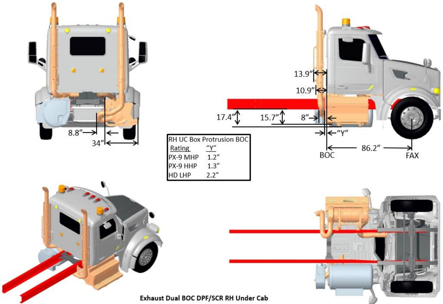
FIGURE 3-54. Exhaust Dual BOC DPF/SCR RH Under Cab
