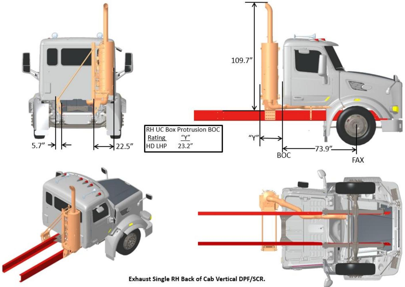
Exhaust Single RH Back of Cab Vertical DPF/SCR.
