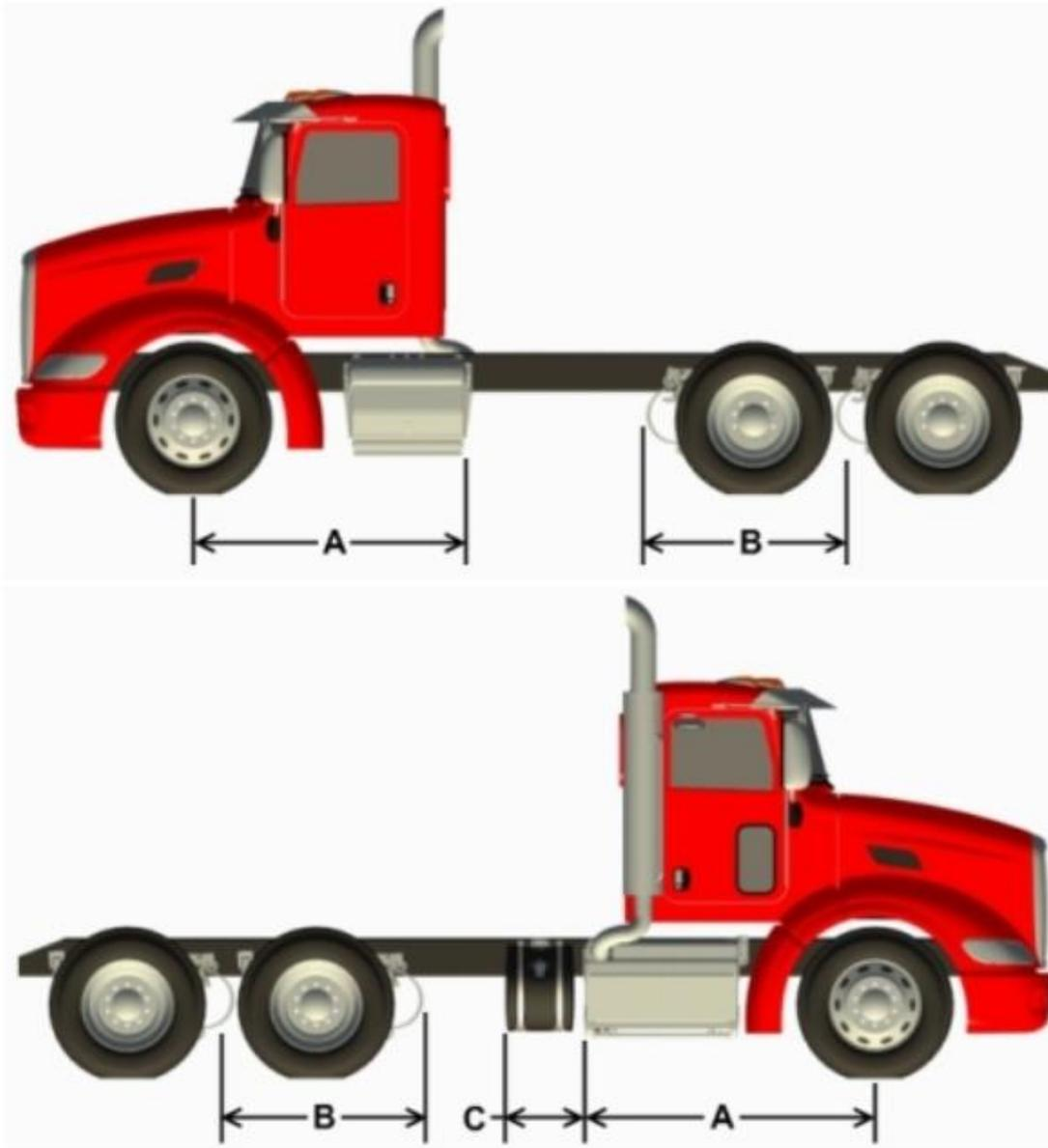
**BASIC FORMULA:** BOC Frame Space = Wheelbase - Dimension A - Dimension C - Dimension B
