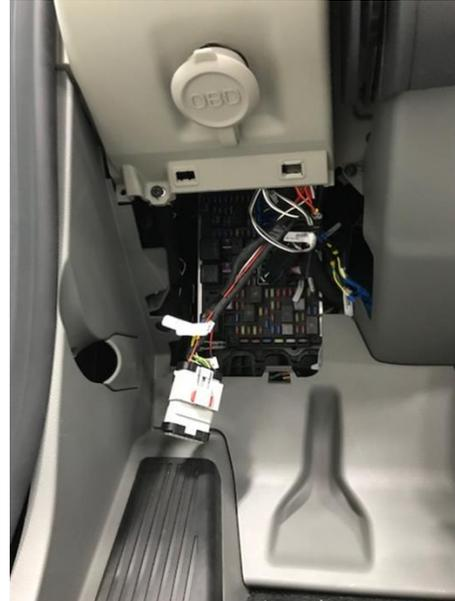
MX PTO CAN functionality may be accessed in the cab through the RP1226 connector and remotely through the body connectors K-CAN (E-3375-021) and B-CAN (DTM06-2S-EP10) Connectors.
