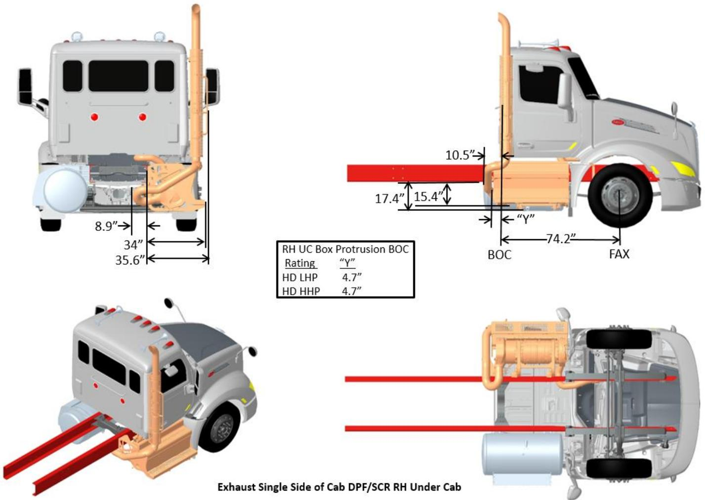
**FIGURE 3-78.** Exhaust Single RH Side of Cab DPF/SCR RH Under Cab
