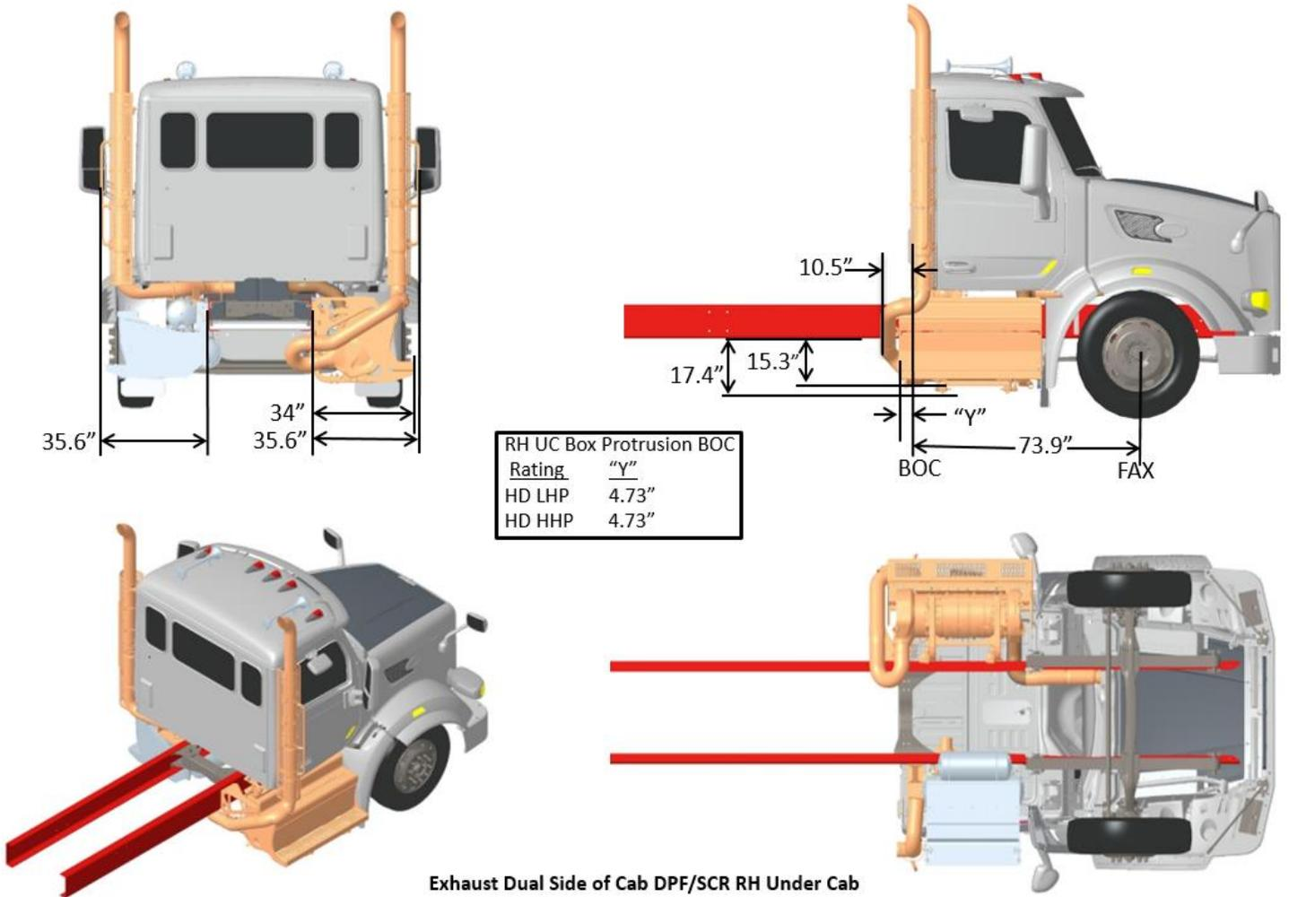
**FIGURE 3-60.** Exhaust Dual SOC DPF/SCR RH Under Cab
