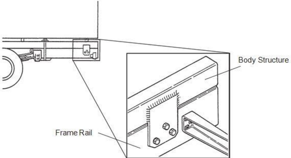
**FIGURE 4-11.** Fishplate Bracket at Rear End of Body
