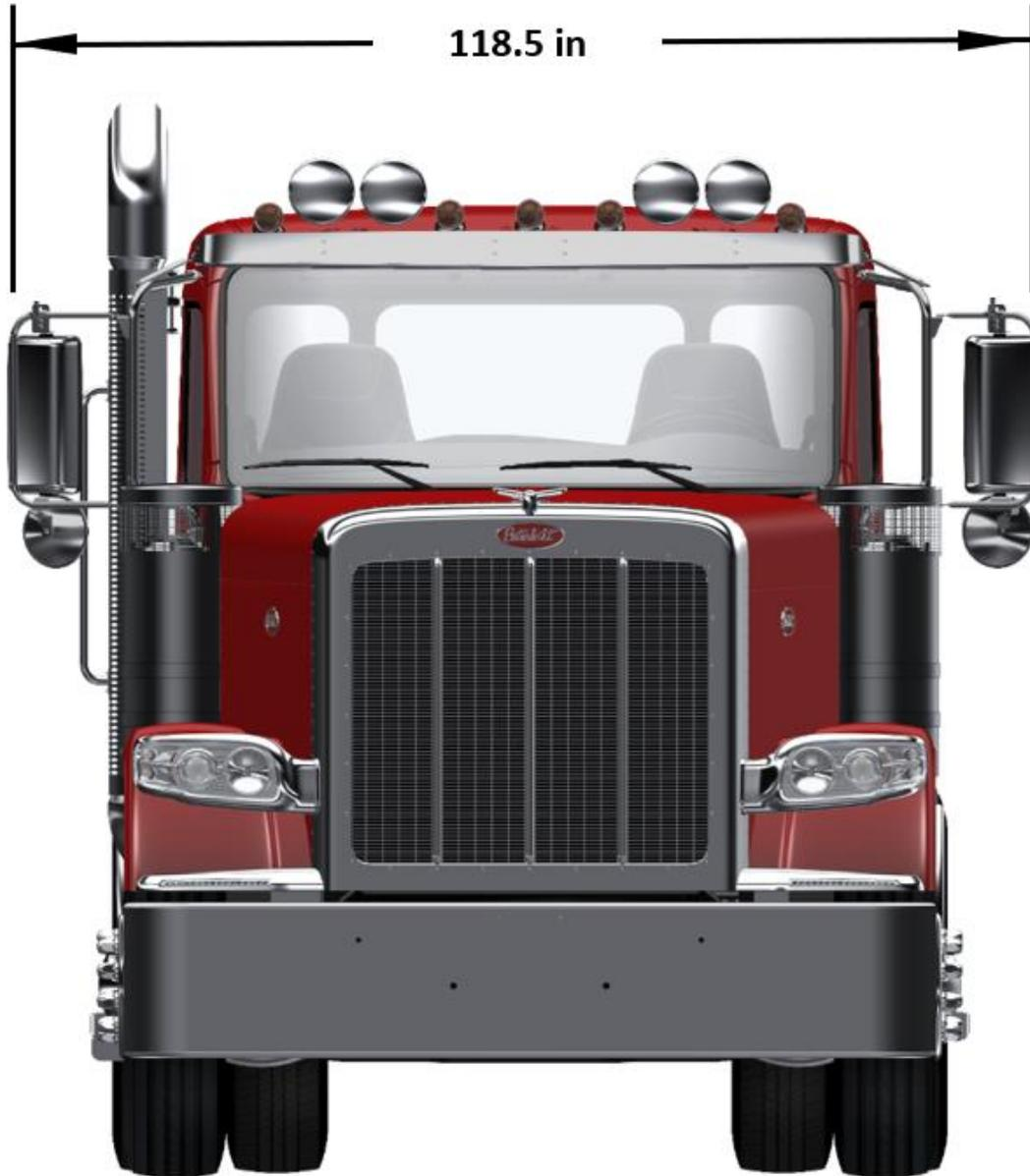
FIGURE 3-3. Model 589-131 Front View – Overall Dimensions
