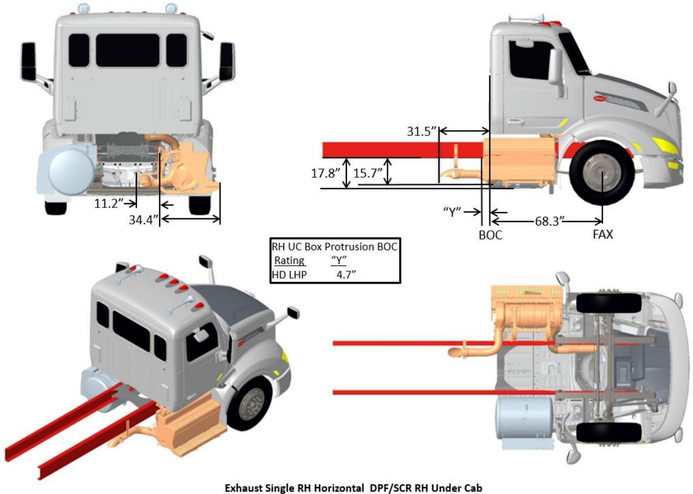
**FIGURE 3-72.** Exhaust Single RH Horizontal DPF/SCR RH Under Cab
