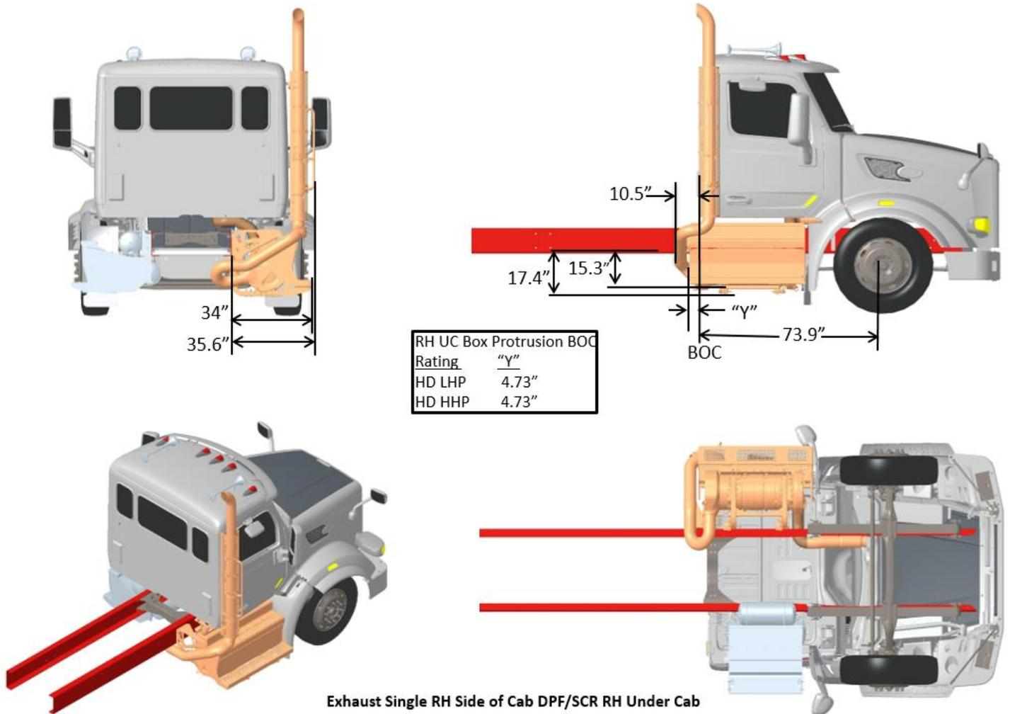
FIGURE 3-57. Exhaust Single RH Side of Cab DPF/SCR RH Under Cab
