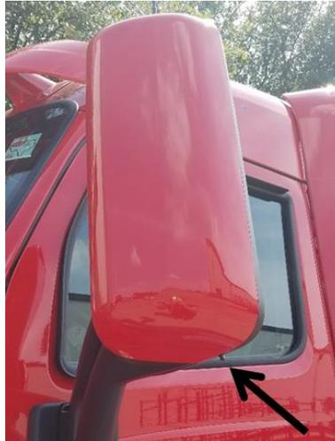
**FIGURE 2-3:** Aerodynamic Mirror OAT Sensor Location
