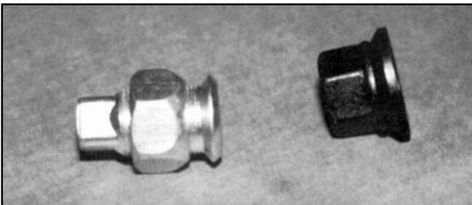
Rounded Ball-seat Type Capnut (Left) and Pilot-mount Two-piece Flange Nut (Right)
