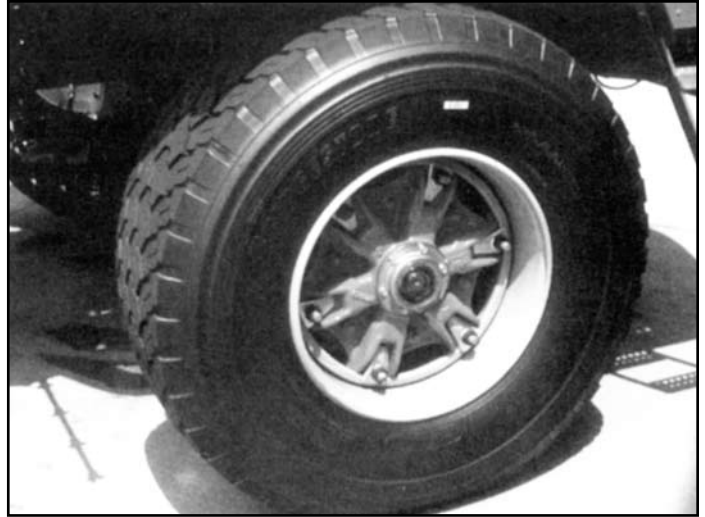
Steel Demountable Rim Mounting System (Six-Spoke)
