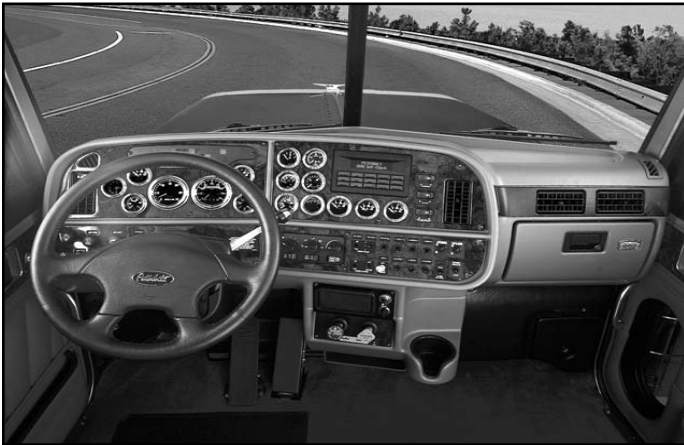
Air Outlets in Cab
