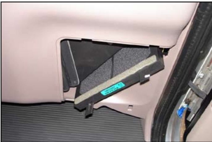
Heating and Air Conditioning Air Filter
