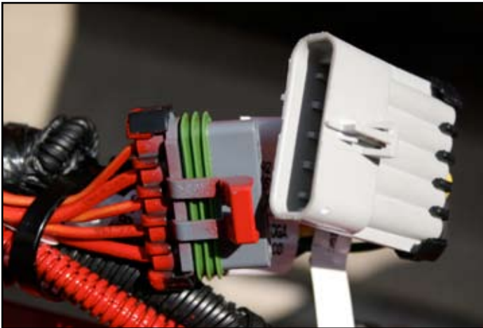
Numbered Wires/Sealed Electrical Connectors
