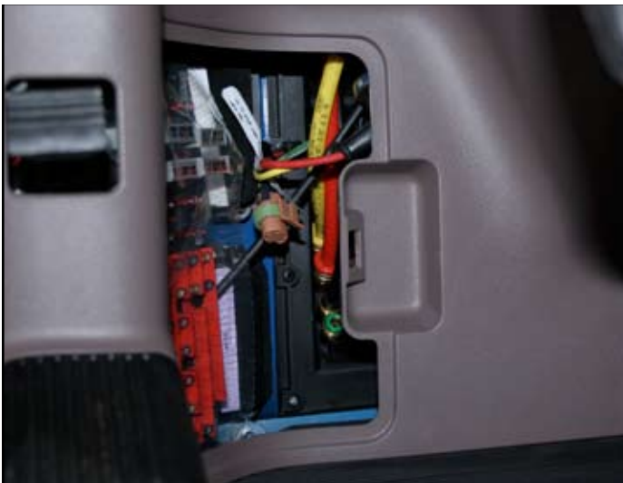
Fuse/Circuit Breaker Panel
