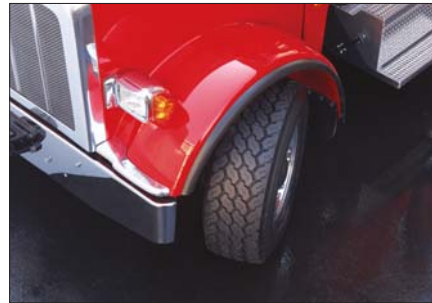
The Model 367 is available in either a SFFA configuration for a smooth ride or a SBFA configuration for more maneuverability and optimized weight distribution.
