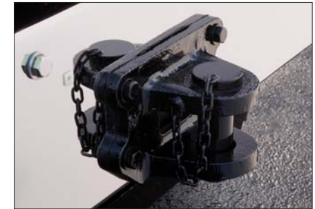
Bumpers on the Model 367 accommodate either a center tow hook configuration or a dual removable pin configuration that meet TMC towing guidelines of 80,000 pounds.
