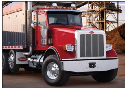
The gently sloped, long-length hood on the Model 367 not only enhances visibility, it allows for a 1,438 square-inch radiator to accommodate engines of up to 600 HP.
