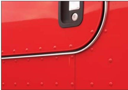
A lightweight, huckbolted, all-aluminum cab with lap seam construction and bulkhead style doors is legendary for toughness and corrosion resistance. It provides years of virtually water-tight performance.
