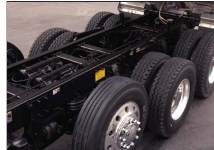
The Model 367 can be spec'd with a variety of heavy duty components including full and partial frame liners, as well as a selection of axles including tandem, tridem and lift-axle options.
