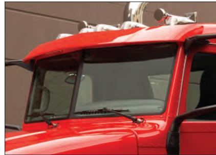
A contoured sunvisor was designed using Computational Fluid Dynamics and extensive wind tunnel testing. A two-piece windshield allows for cost-efficient glass replacement.
