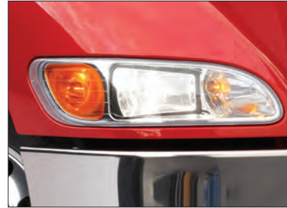
The sloped hood and high-intensity forward lighting system provide improved visibility. The tough Lexan® lens is impact resistant and no special tools are required for lamp adjustment or bulb replacement.
