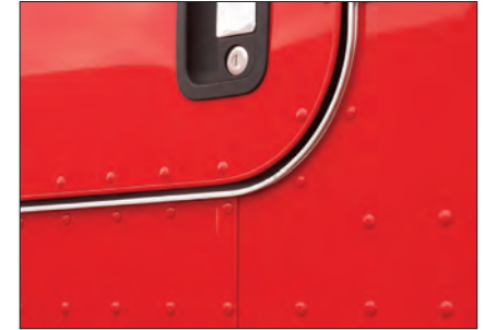
A lightweight all-aluminum cab with huckbolt fasteners, lap seam construction and bulkhead style doors is the leader in toughness, corrosion resistance and water-tight performance.
