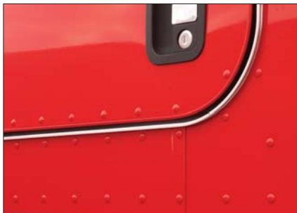
A lightweight all-aluminum cab is huckbolted with lap seam construction and bulkhead style doors for toughness and corrosion resistance. It offers years of virtually water-tight, rattle-free performance.
