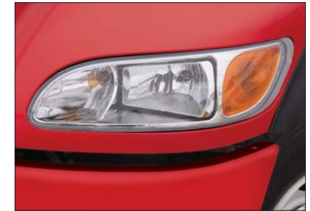
An impact-resistant Lexan® lens safeguards a high-intensity forward lighting system integrated into the fender. No special tools are needed for lamp adjustment or bulb replacement.
